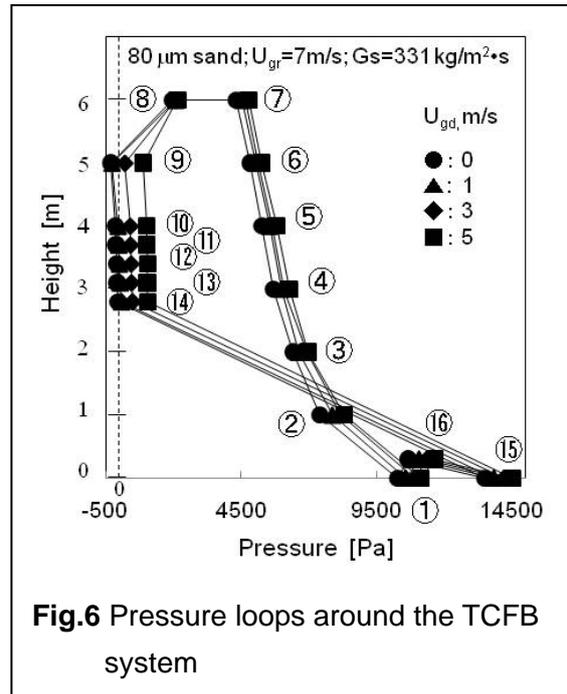
**Fig.6** Pressure loops around the TCFB system
