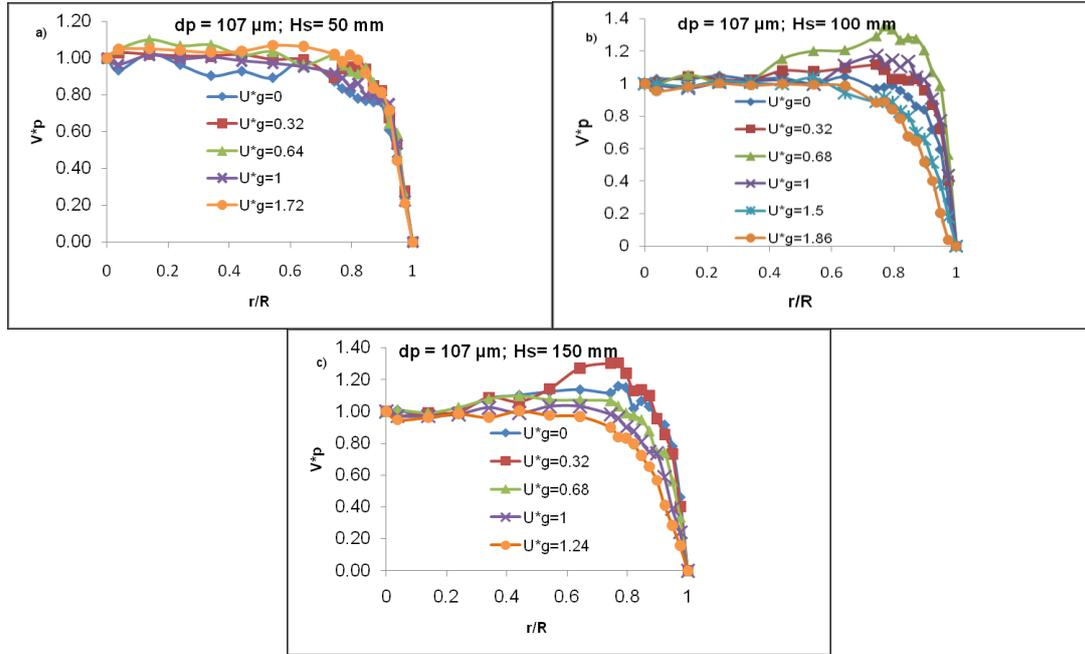
Fig.2. Evolution of the dimensionless axial particle velocity  $V_p^*$  as function of  $U_g^*$ .  $d_p=107 \mu\text{m}$ ;  $z/H=0.7$ : a)  $H_s=50 \text{ mm}$ , b)  $H_s=100 \text{ mm}$ , c)  $H_s=150 \text{ mm}$ .
