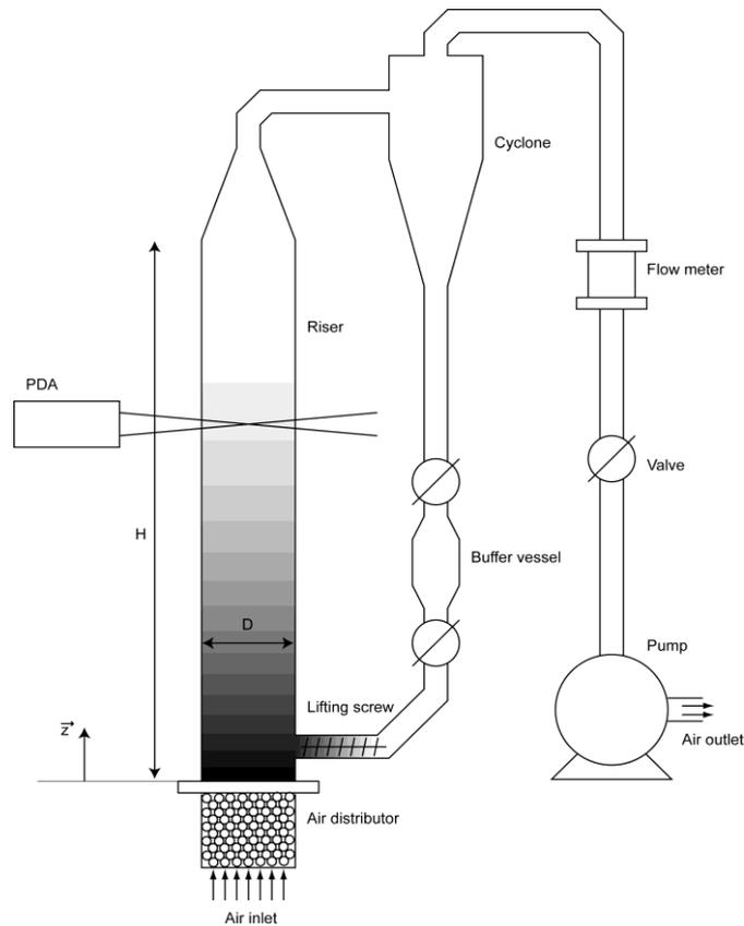
Fig.1. Schematic diagram of the circulating fluidized bed set up
