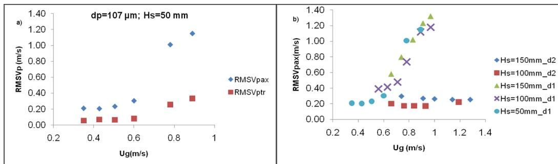
Fig.5. Standard deviation of mean particle velocity as a function of  $U_g$  at the center riser ( $r/R=0$ ): a) Comparison of  $RMSV_{pax}$  and  $RMSV_{ptr}$ ; b)  $RMSV_{pax}$  for both distribution 1 and 2.
