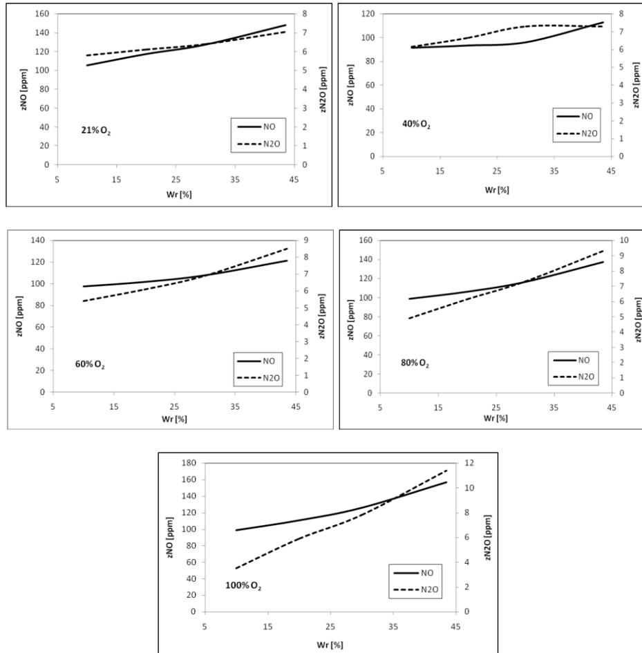
Fig.2. NO and N<sub>2</sub>O concentration in dry flue gas as a function of moisture content in fuel for different oxygen content in the inlet gas of O<sub>2</sub>/N<sub>2</sub>
