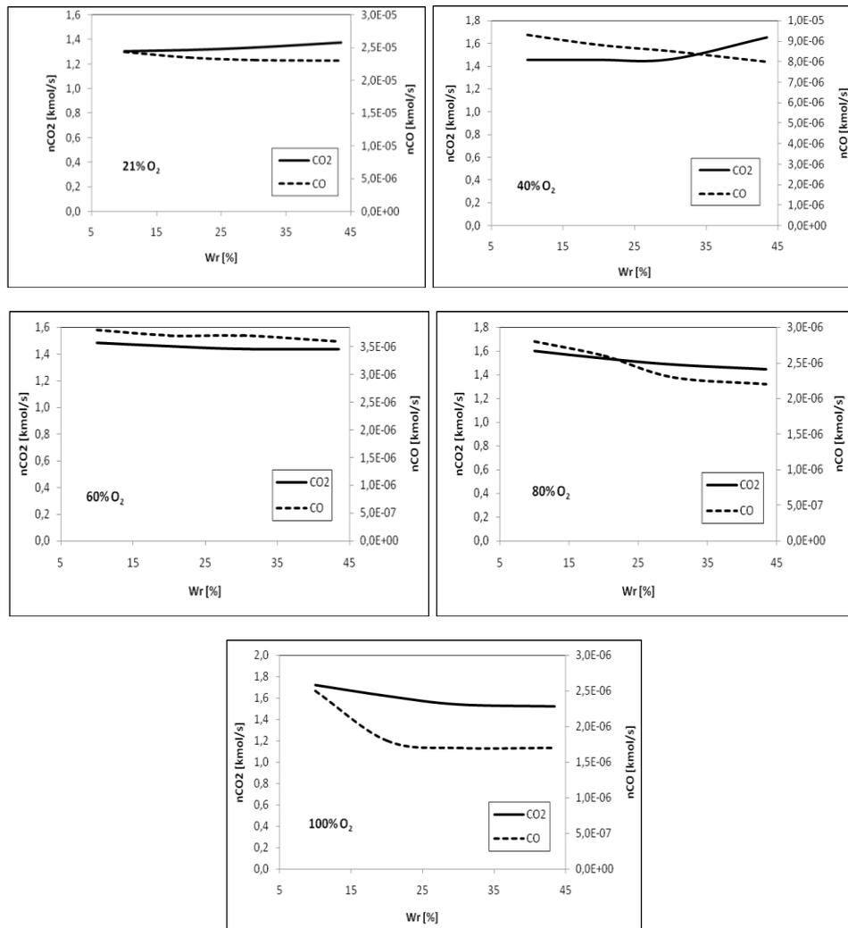
Fig.3. CO<sub>2</sub> and CO flux in dry flue gas as a function of moisture content in fuel for different oxygen content in the inlet gas of O<sub>2</sub>/N<sub>2</sub>
