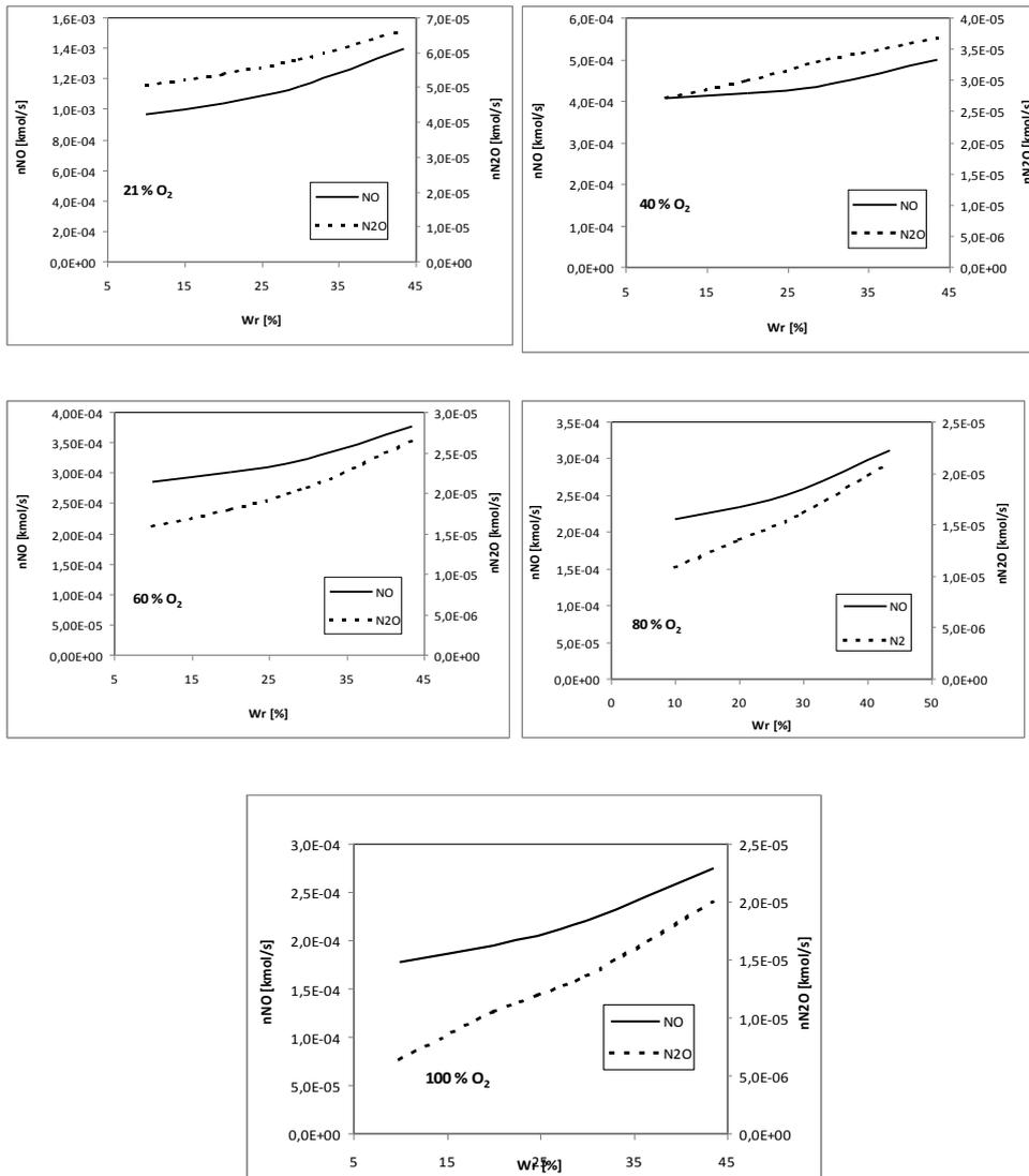
Fig.4. NO and N<sub>2</sub>O flux in dry flue gas as a function of moisture content in fuel for different oxygen content in the inlet gas of O<sub>2</sub>/N<sub>2</sub>
