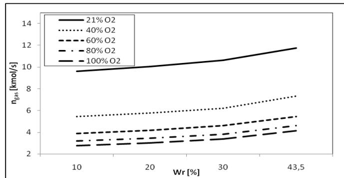
Fig.5. Flux of wet flue gas as a function of moisture content in fuel for different oxygen content in the inlet gas of O<sub>2</sub>/N<sub>2</sub>
