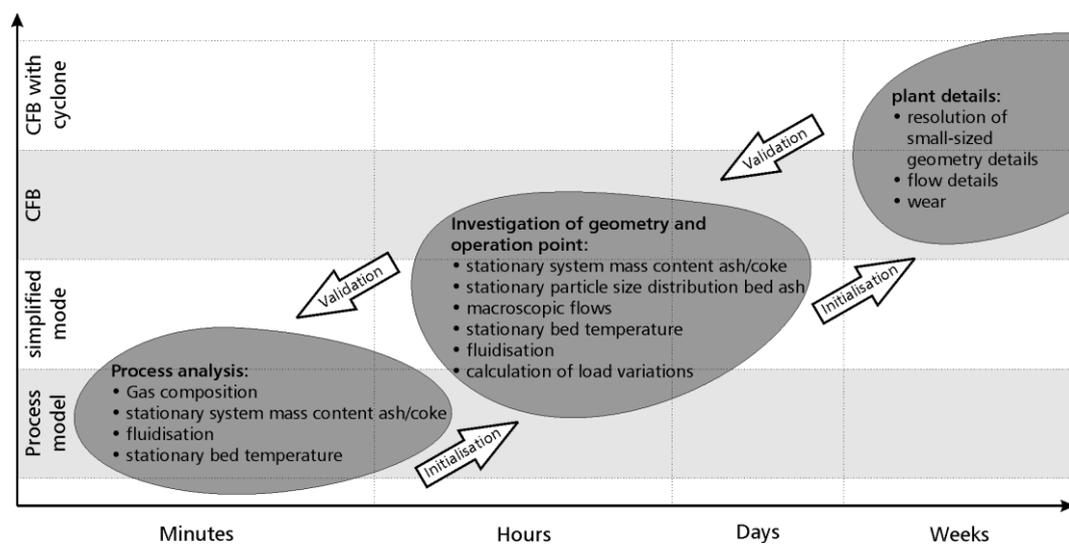
Figure 1: Flow of information with the multi-level simulation concept, Comparison of level of detail and simulation time and effort
