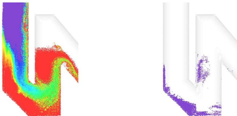
Figure 6: Sand particles coloured by residence time (left-hand side), blue particles have a short, red particles a long residence time. Particles selected by their momentary velocity, only particles slower than 1 cm/s are shown (right-hand side).
