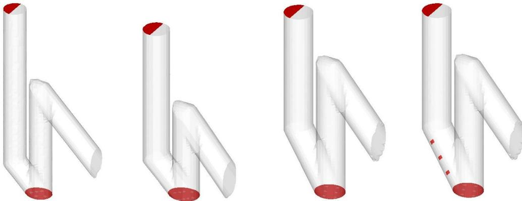
Figure 5: Evolution of basic siphon design from first design (leftmost) over a version with increased diameter (left-center), a version with increased slope angle (right-center) to version ready for detail optimisation (right).
