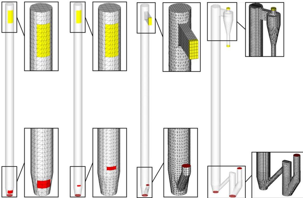
Figure 2: Representation of employed geometry and the computational grid in the process model (leftmost), the simplified model (left-hand side), the detailed model (right-hand side) and the complete model (rightmost)
