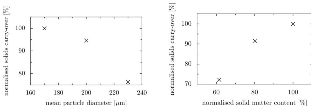
Figure 4: Showcase plots of the effect of influencing variables on solids carry-over: solids carry-over against mean particle diameter of bed material (left-hand side) and against amount of solids contained in the riser of the CFB (right-hand side).
