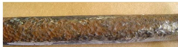
Fig. 1-b) External Tube Corrosion
