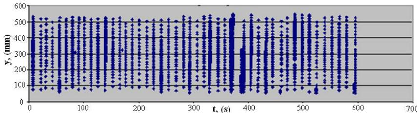
Fig.2. Illustration of the axial (vertical) component of the tracer movement at  $U$  of  $2.55 \text{ m s}^{-1}$  and  $G$  of  $77.5 \text{ kg m}^{-2} \text{ s}^{-1}$  within the geometric limits of the detectors
