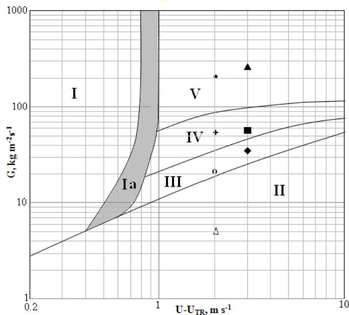
Fig.7. Modes of operation of a CFB riser, expressed as  $G$  vs  $U-U_r$  depending on
