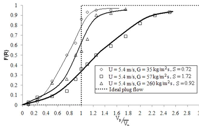
Fig. 8: Solids flow behaviour in the riser at  $U = 5.4 \text{ m s}^{-1}$  but increasing  $G$  from  $35 \text{ kg m}^{-2} \text{ s}^{-1}$  to  $260 \text{ kg m}^{-2} \text{ s}^{-1}$
