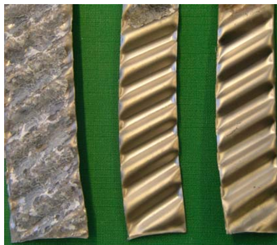
Fig. 12 The effect of heat treatment and electrochemical cleaning on AISI 316L fouled by the calcium carbonate process. From left to right: the fouled sample, sample after heat treatment and electrochemical cleaning, and the sample resulting from electrochemical cleaning only.
