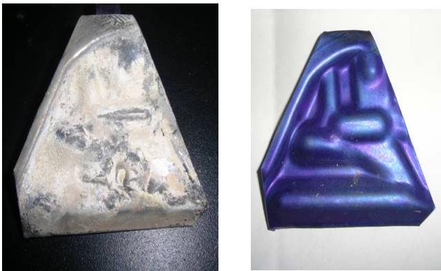
Fig. 6 Sample scraped due to excess fouling before and after cleaning using pulse current, 10 w-% H 2 SO 4 + 1000 ppm citric acid, T= 60 °C, pulse current 5 min.
