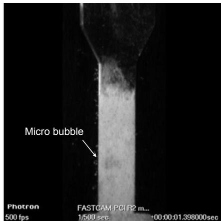
Figure 5. A rising bubble in the 3mmX3mm microfluidic channel
