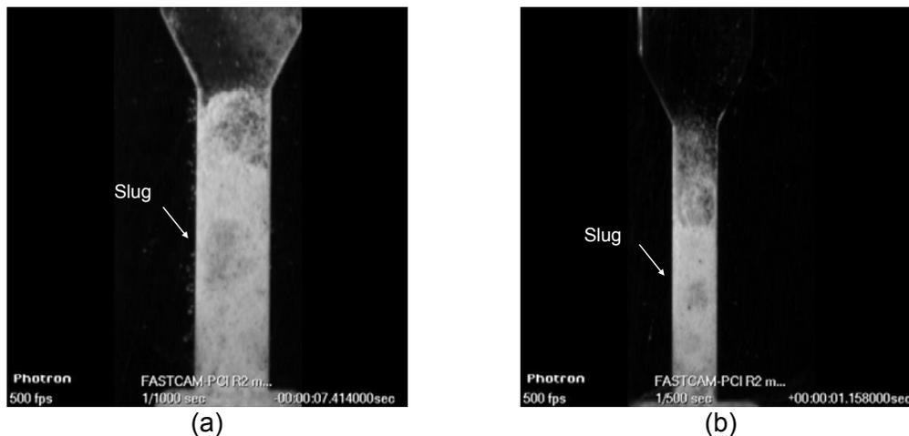
Figure 7. Snapshots of slugs in the microfluidic channels: (a)  $U_g=55$  mm/s; channel size=3mmX3mm; (b)  $U_g=58$  mm/s; channel size=2mmX3mm
