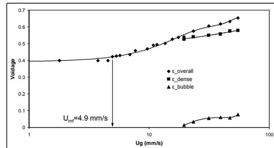
Figure 4. Fluidization map for the 3mmX3mm microfluidic channel
