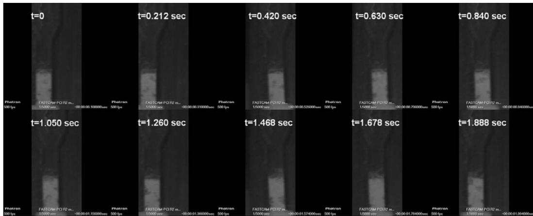
Figure 8 Snapshots of gas-solid fluidization in a 3mmX3mm microfluidic channel in the centrifugal force field:  $\omega=287$  r/m;  $U_g=15.5$  mm/s
