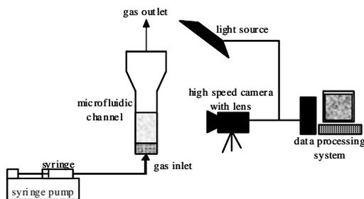
Figure 1. Schematic diagram of the microfluidic gas-solid fluidization system
