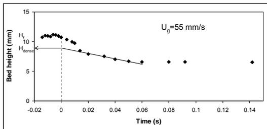
Figure 3. Dynamic bed height in the 3mmX3mm microfluidic channel from the bed collapse experiment
