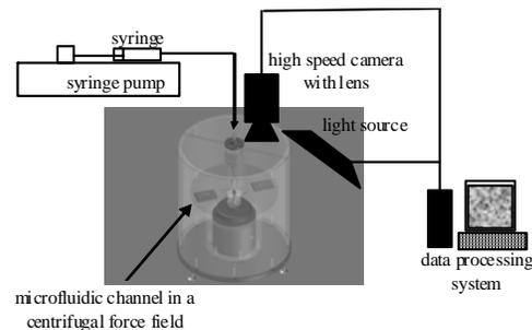
Figure 2. Microfluidic gas-solid fluidization system in a centrifugal force field
