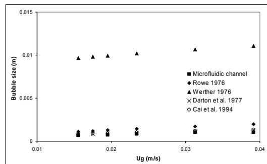
Figure 6. Comparison of bubble sizes in the 3mmX3mm microfluidic channel and
