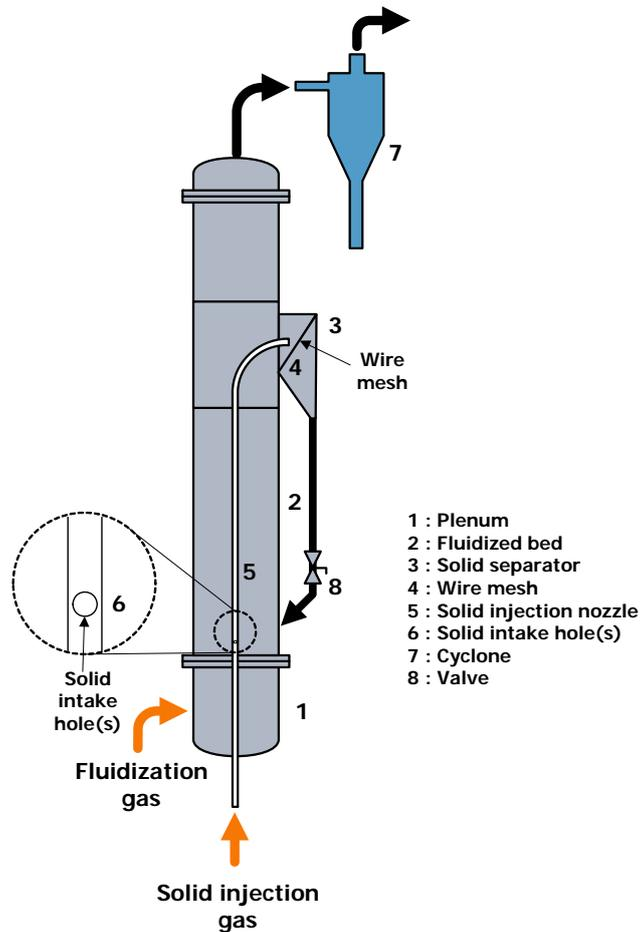
Figure 1. Schematic of solid separation test apparatus.
