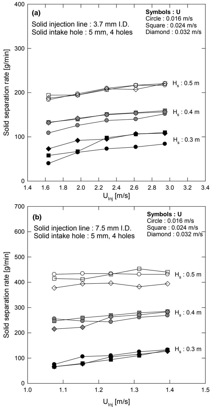
Figure 2. Solid separation rate versus solid injection velocity.
