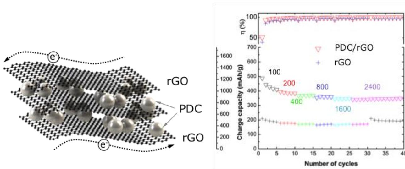
Figure 1 – Schematic of PDC/rGO composite paper. PDC provides high lithiation capacity while reduced graphene oxide (rGO) acts as a flexible support and electron conductor.
