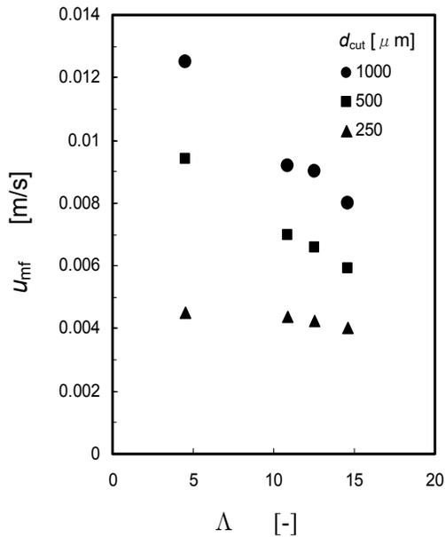
Figure 4 Effect of vibration on  $u_{mf}$  for different  $d_{cut}$
