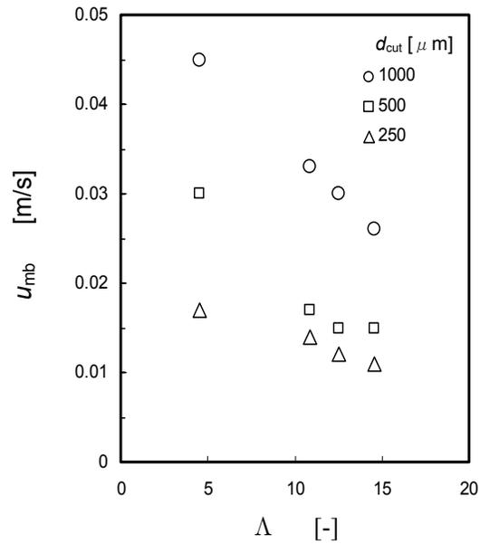
Figure 5 Effect of vibration on  $u_{mb}$  for different  $d_{cut}$
