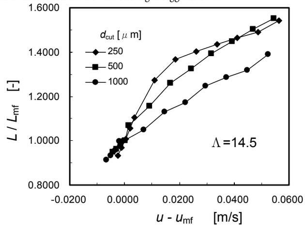
Figure 6 Comparison of bed expansion ratio ( $\Lambda = 14.5$ )
