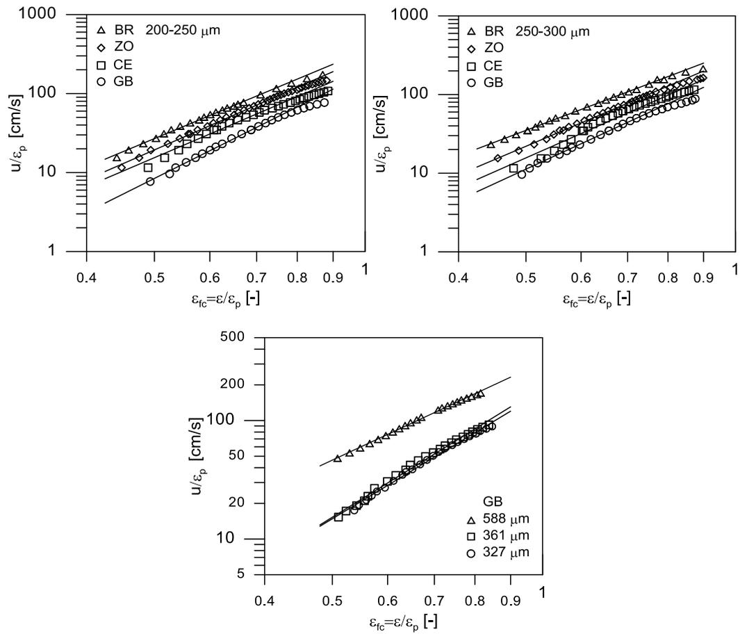
**Fig.4 - Expansion diagrams of the confined fluidized beds.**
