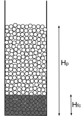
**Fig.1 - Sketch of the confined fluidized bed.**
