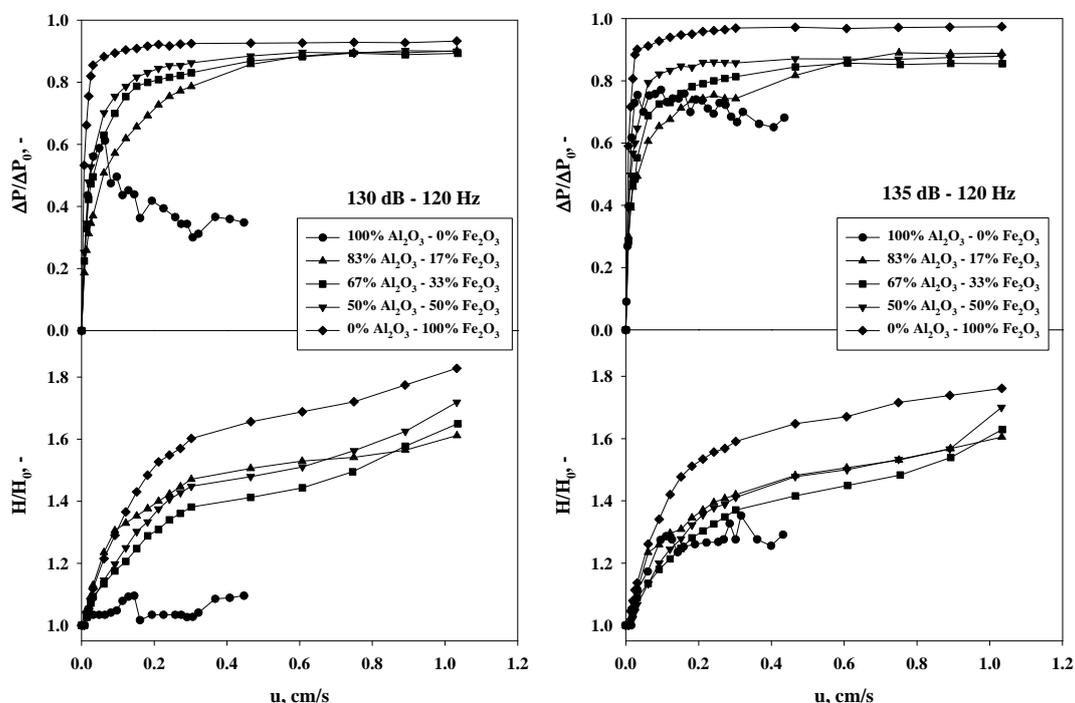
Figure 2. Dimensionless pressure drop ( $\Delta P/\Delta P_0$ ) and bed expansion ratio ( $H/H_0$ ) as a function of superficial gas velocity during aeration with application of different acoustic fields for binary mixtures of  $\text{Al}_2\text{O}_3$  and  $\text{Fe}_2\text{O}_3$ .
