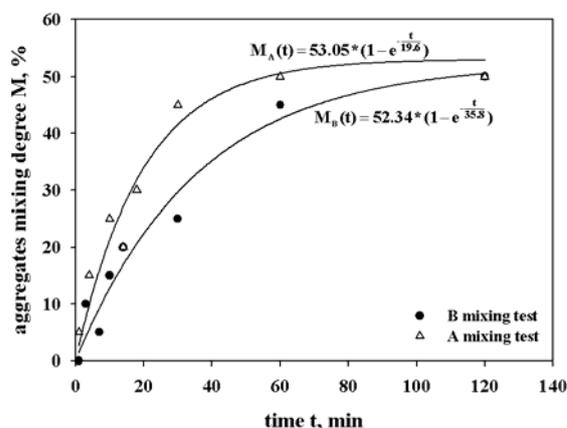
Figure 5. Time dependence of aggregates mixing degree for A and B mixing tests.
