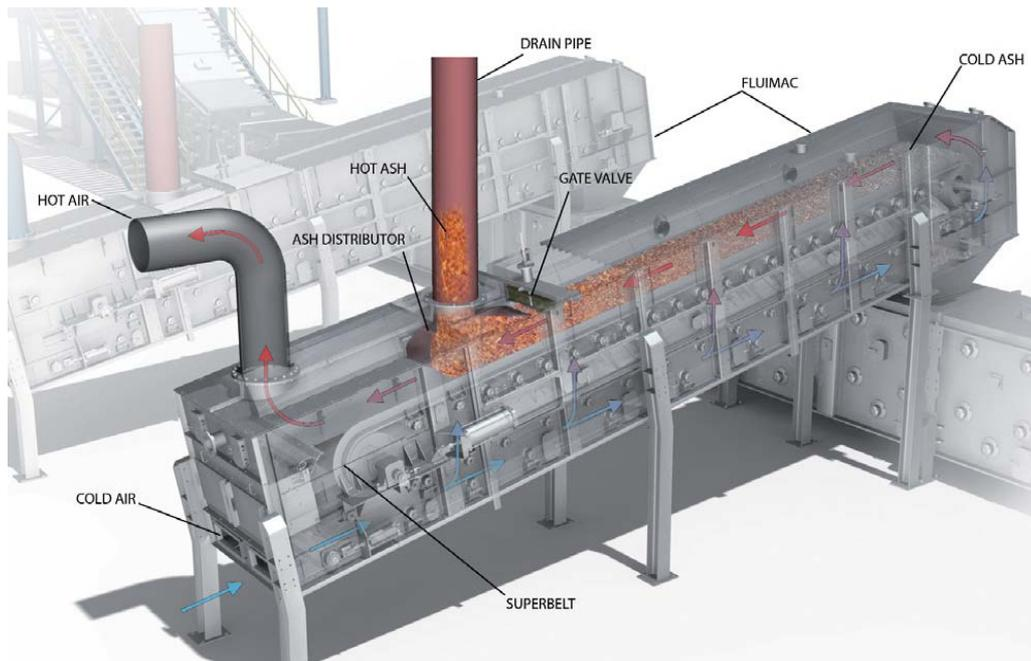
**Figure 2: FluiMAC<sup>®</sup> ash extraction and cooling**
