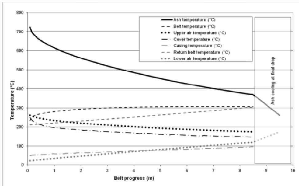
Figure 3: Ash cooling simulation results
