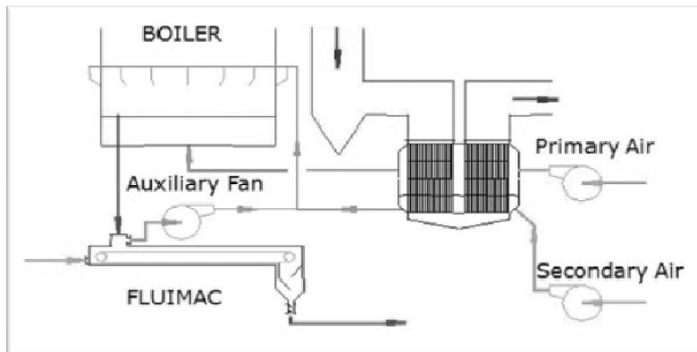
Figure 4: Yeosu#2 heat recovery scheme
