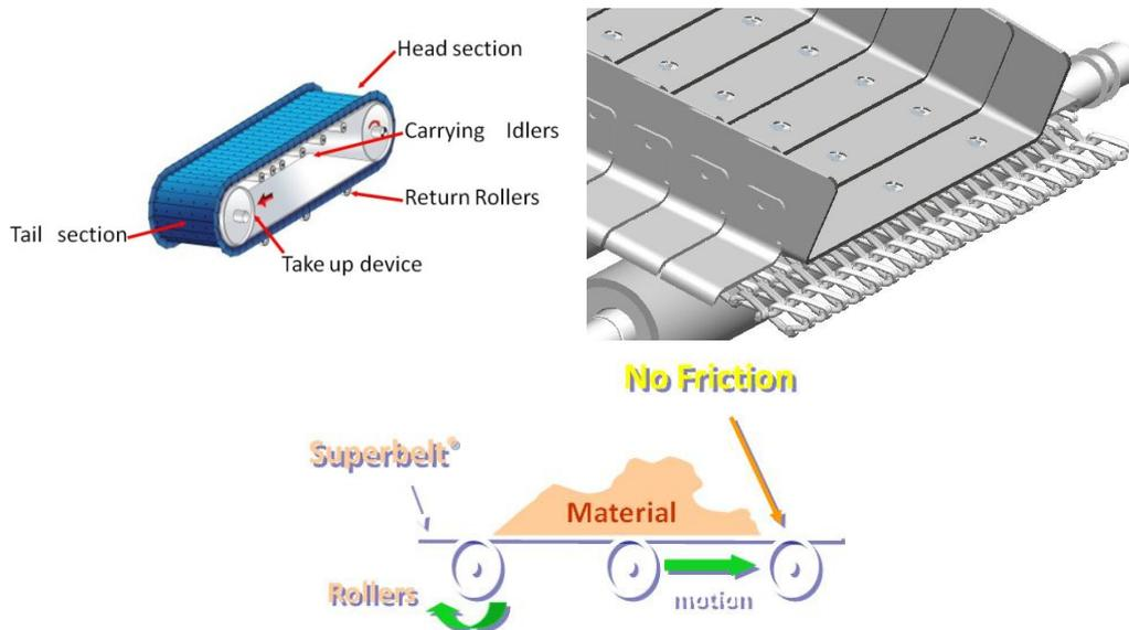
**Figure 1: Superbelt<sup>®</sup> working concept**
