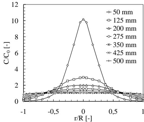
Fig. 6: Radial dimensionless tracer gas concentration profiles  $C/C_0$ ;  $U_G = 0.46$  m/s,  $U_{Jet} = 60.13$  m/s,  $d_p = 732$   $\mu$ m,  $\rho_S = 2480$  kg/m<sup>3</sup>,  $h_{bed} = 700$  mm
