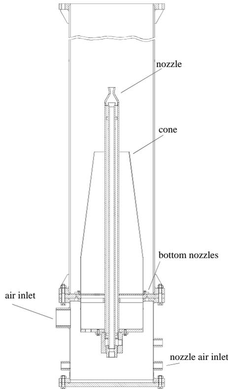
Fig. 1: Fluidized bed reactor model
