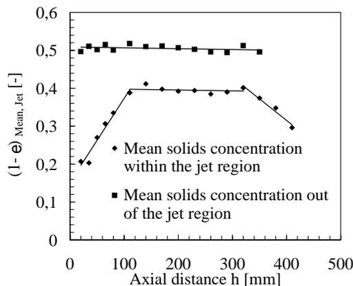
Fig. 5: Dependency of mean solids concentration within and outside the jet region on axial distance  $h$ ;  $U_G = 0.46$  m/s,  $U_{Jet} = 60.13$  m/s,  $d_p = 732$   $\mu$ m,  $\rho_s = 2480$  kg/m<sup>3</sup>,  $h_{bed} = 700$  mm
