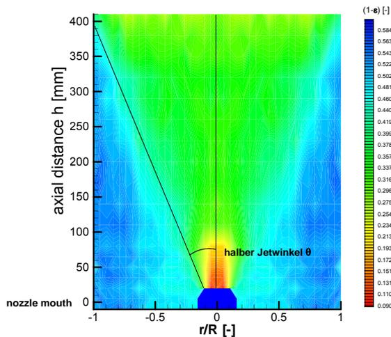
Fig. 3: Solids concentration distribution;  $U_G = 0.46$  m/s,  $U_{Jet} = 60.13$  m/s,  $d_p = 732$   $\mu$ m,  $\rho_s = 2480$  kg/m<sup>3</sup>,  $h_{bed} = 700$  mm
