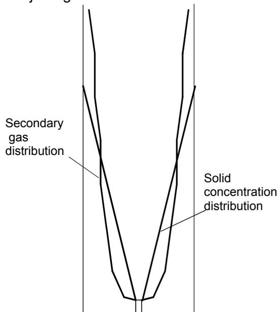
Fig. 9: Boundaries of jet region on the basis of different parameters;  $U_G = 0.47$  m/s;  $U_{Jet} = 60.13$  m/s;  $d_p = 732$   $\mu$ m;  $\rho_S = 2480$  kg/m<sup>3</sup>;  $h_{bed} = 700$  mm
