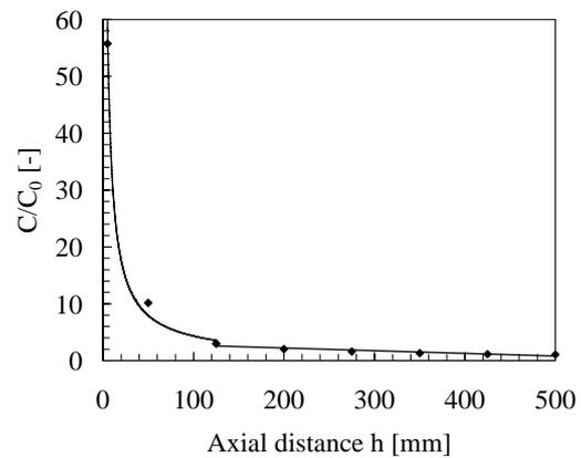
Fig. 8: Dimensionless jet gas concentration  $C/C_0$  at the radial position  $r/R = 0$  depending on the axial distance  $h$ ;  $U_G = 0.46$  m/s,  $U_{Jet} = 60.13$  m/s,  $d_p = 732$   $\mu$ m,  $\rho_S = 2480$  kg/m<sup>3</sup>,  $h_{bed} = 700$  mm
