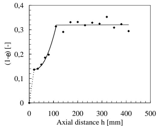
Fig. 4: Solids concentration at the radial position  $r/R = 0$  against the axial distance  $h$ ;  $U_G = 0.46$  m/s,  $U_{Jet} = 60.13$  m/s,  $d_p = 732$   $\mu$ m,  $\rho_s = 2480$  kg/m<sup>3</sup>,  $h_{bed} = 700$  mm
