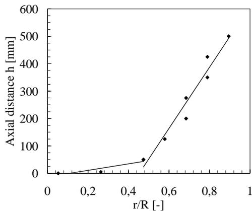
Fig. 7: Boundary of jet region on the basis of jet gas distribution;  $U_G = 0.46$  m/s,  $U_{Jet} = 60.13$  m/s,  $d_p = 732$   $\mu$ m,  $\rho_S = 2480$  kg/m<sup>3</sup>,  $h_{bed} = 700$  mm
