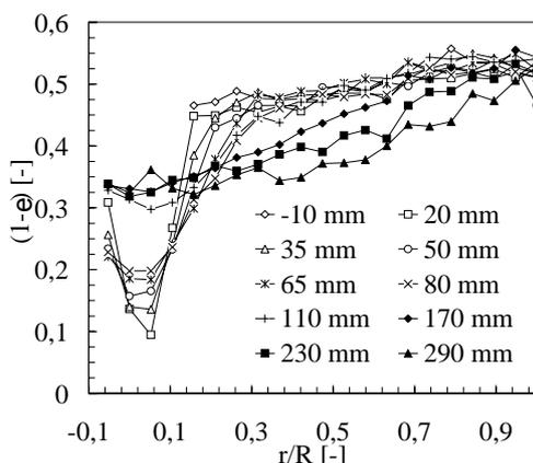
Fig. 2: Radial solids concentration profiles for different axial distances  $h$  from the nozzle mouth;  $U_G = 0.46$  m/s,  $U_{Jet} = 60.13$  m/s,  $d_p = 732 \mu\text{m}$ ,  $\rho_S = 2480 \text{ kg/m}^3$ ,  $h_{bed} = 700$  mm
