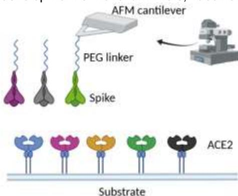
Figure 1: Schematic principle of atomic force microscopy (AFM) in our setup. The spike protein/glycomutants is linked to the tip of the cantilever to study interaction forces with the ACE2 glycomutants (both indicated by color codes). These variants are immobilized on the substrate.
