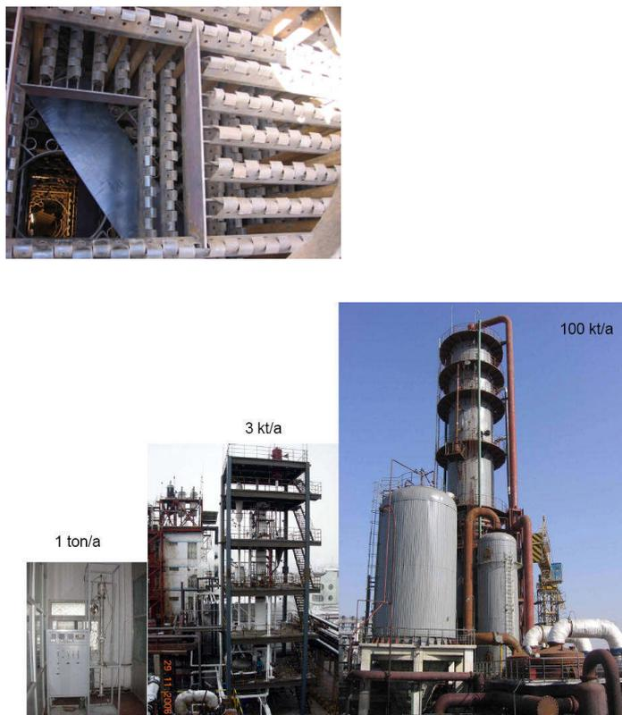
**Fig. 8.** Top: Internal structured fluidized bed reaction; Bottom: Multistage fluidized bed reactor for VCM production scale-up process: Left: small hot model test unit; Middle: 3 kT/a pilot plant; Right: 100kT/a multistage fluidized bed CVM unit
