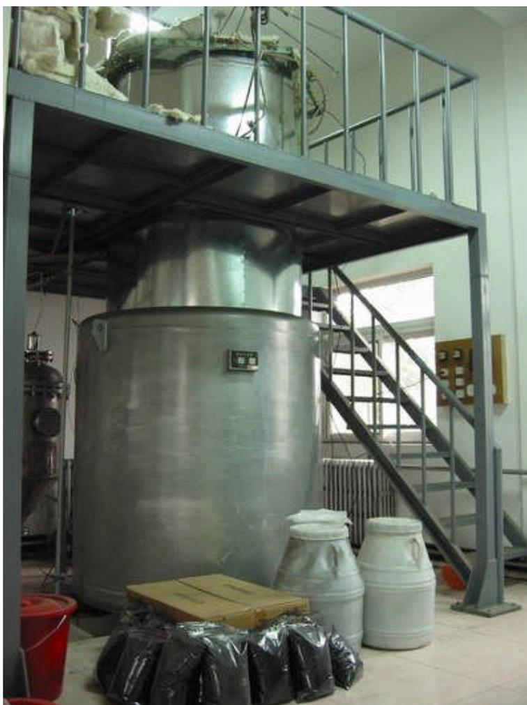
Fig. 4. The pilot plant facility for MWCNT production.<sup>[1]</sup>
