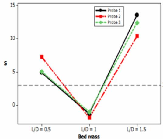
**Figure 4** S-values of comparisons between vibration signatures of different Aspect ratio
