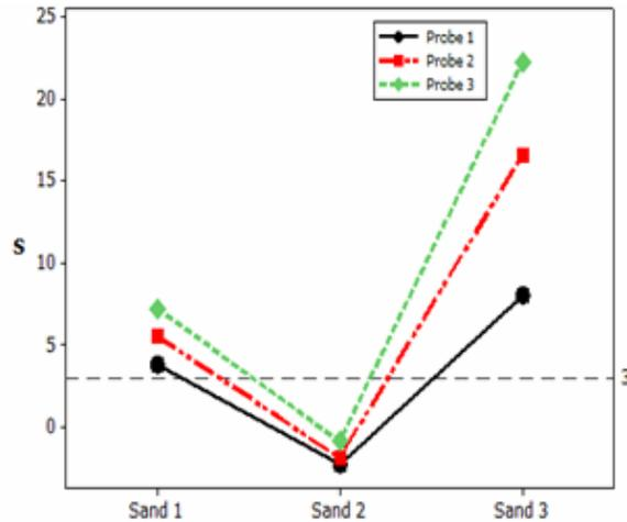
**Figure 5** S-values of comparisons between vibration signatures of different size of sand
