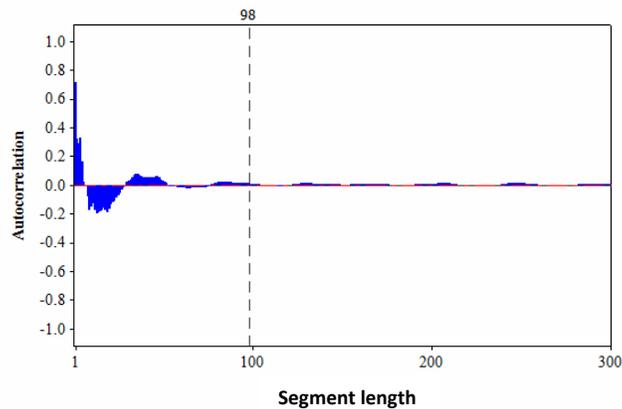
Figure 2 Autocorrelation function of a sample vibration signatures
