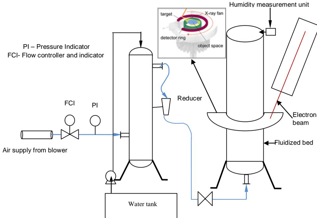
Figure 1: Sketch of X-ray tomography on fluidized beds; experimental setup.
