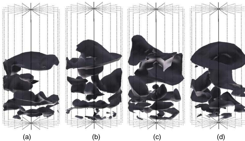
**Figure 3:** Simulated 3-D contours plot of bubbles for LLDP particles fluidizing at  $1.5U_{mf}$  (a) 2.0 s (b) 4.0 s (c) 6.0 s (d) 8.0 s from the start of fluidization.
