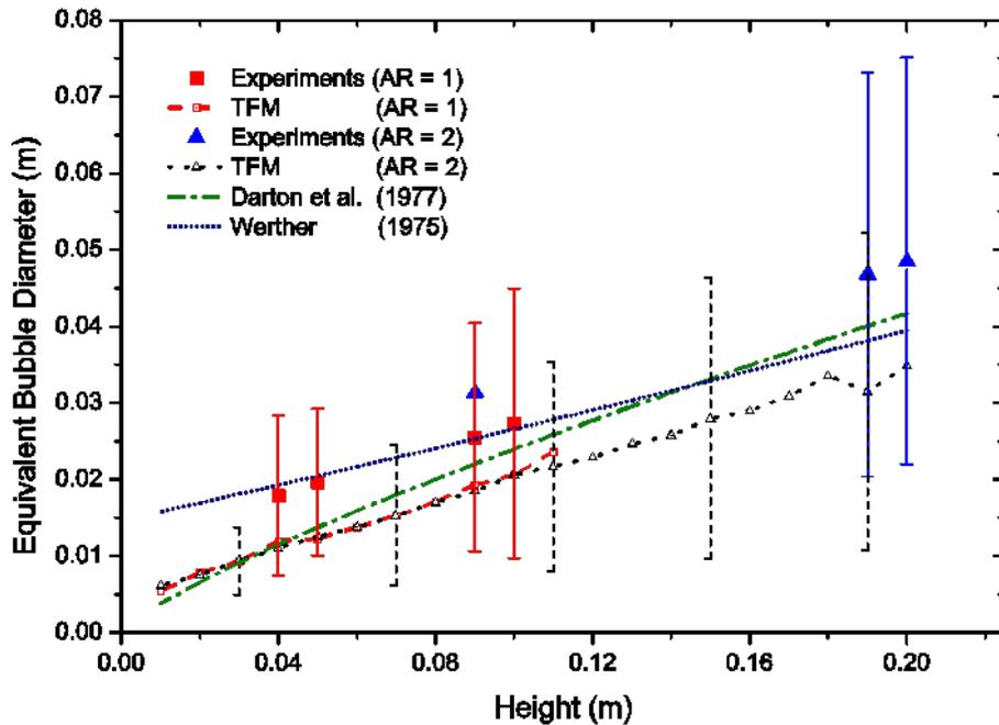
**Figure 4:** Time-averaged equivalent bubble diameter at different height in the fluidized bed, for fluidization of LLDP particles at  $1.5U_{mf}$ . Vertical bars represent standard deviation in the measured (solid vertical bar) and TFM (dash vertical bar) bubble diameter.
