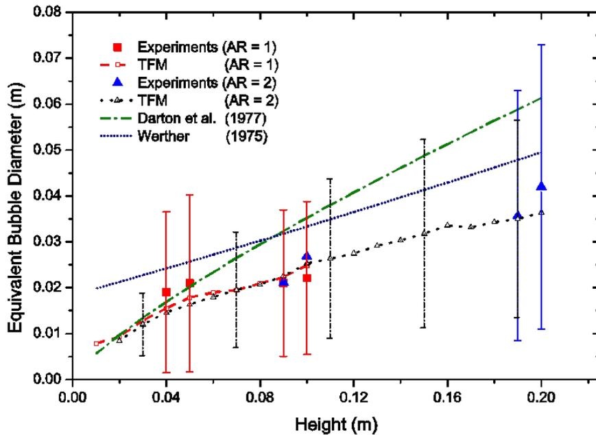
**Figure 5:** Time-averaged equivalent bubble diameter at different height in the fluidized bed, for fluidization of glass particles at 1.5Umf. Vertical bars represent standard deviation in the measured (solid vertical bar) and TFM (dash vertical bar) bubble diameter.
