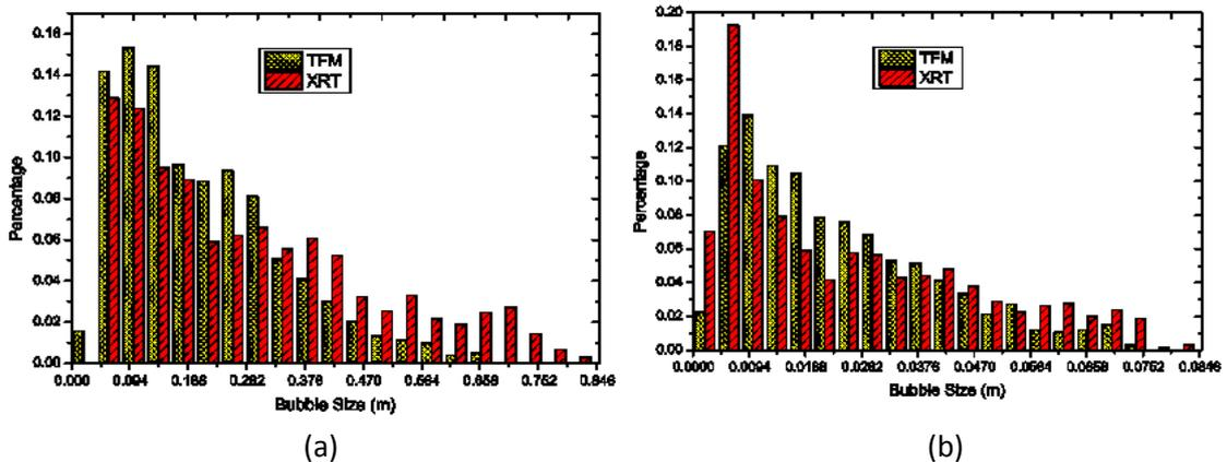
**Figure 6:** Distribution of bubbles for different size group at the height of 10 cm from the gas distributor, fluidizing at 1.5Umf. (a) LLDP particles, (b) Glass particles.
