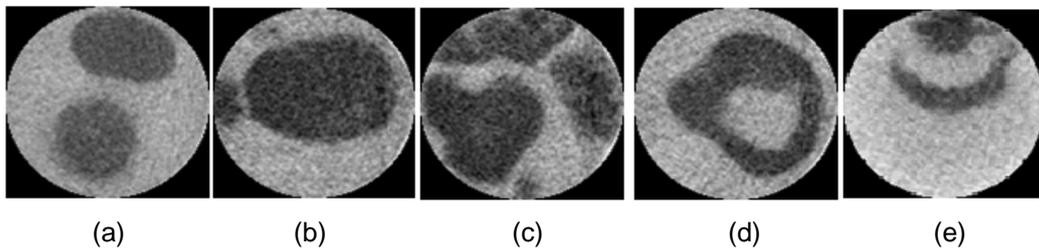
**Figure 2:** Different shapes of bubbles observed experimentally in the cross-sectional planes during fluidization. (a) Small spherical bubbles, (b) large spherical bubbles, (c) irregular bubbles, (d) spherical cap bubbles, and (e) arcs (wakes).
