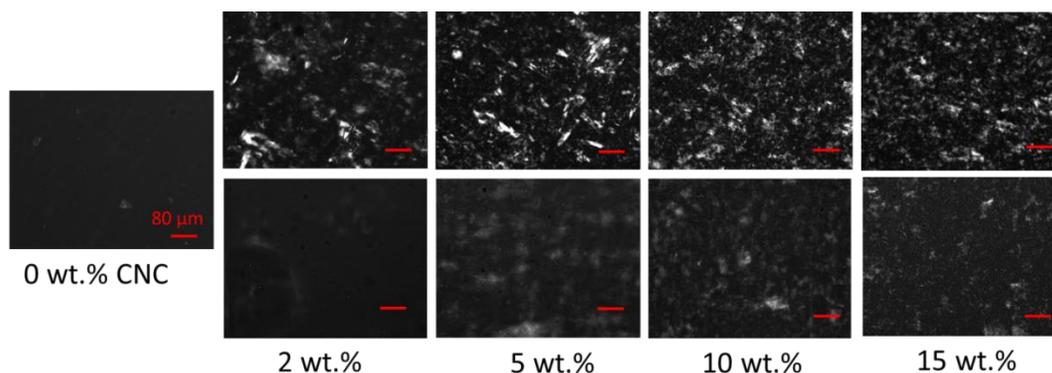
Figure 1 – Polarized light microscopy images of CNC/epoxy composites. Top: one-step mixing, bottom: two-step mixing [1, 2]. Lesser birefringence was observed for samples produced by two-step mixing, indicating that CNCs domains were smaller.
