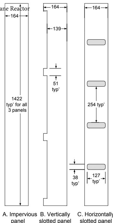
A. Impervious panel B. Vertically slotted panel C. Horizontally slotted panel
