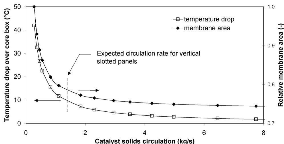
Figure 7: Effect of solids circulation on the core reactor temperature drop and relative membrane area. Conditions: 50 Nm<sup>3</sup>/h H<sub>2</sub>, steam:carbon molar ratio = 3, methane feed = 25 Nm<sup>3</sup>/h, reactor pressure 1,500 kPa, feeds preheated to 650°C
