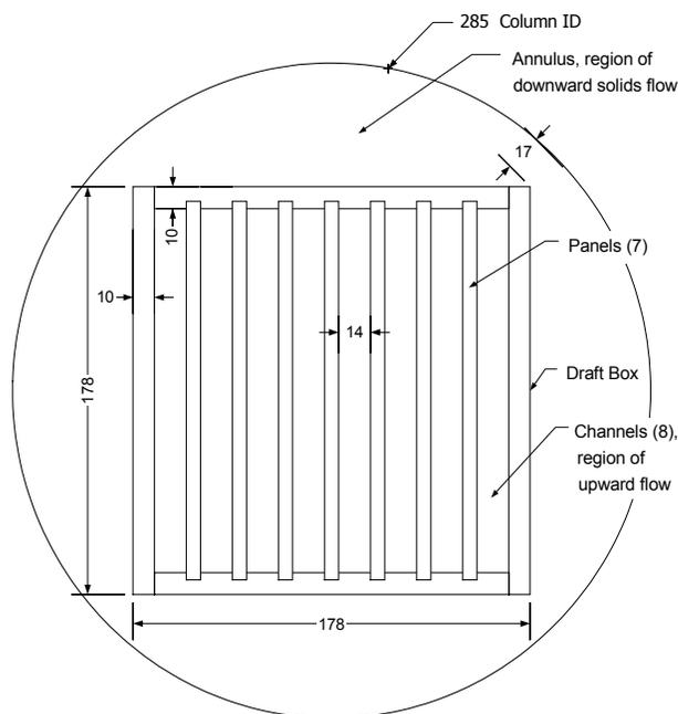
Figure 3: Cold model plan (dimensions in mm)
