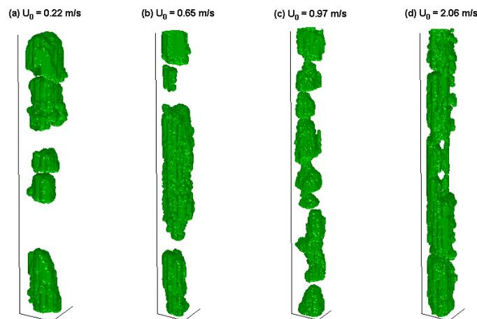
**Figure 6:** 3-D reconstruction of the void shapes at 400 mm above the distributor for the (a) bubbling regime, (b) bubble-turbulent regime transition, (c) turbulent regime and (d) fast fluidization regime.
