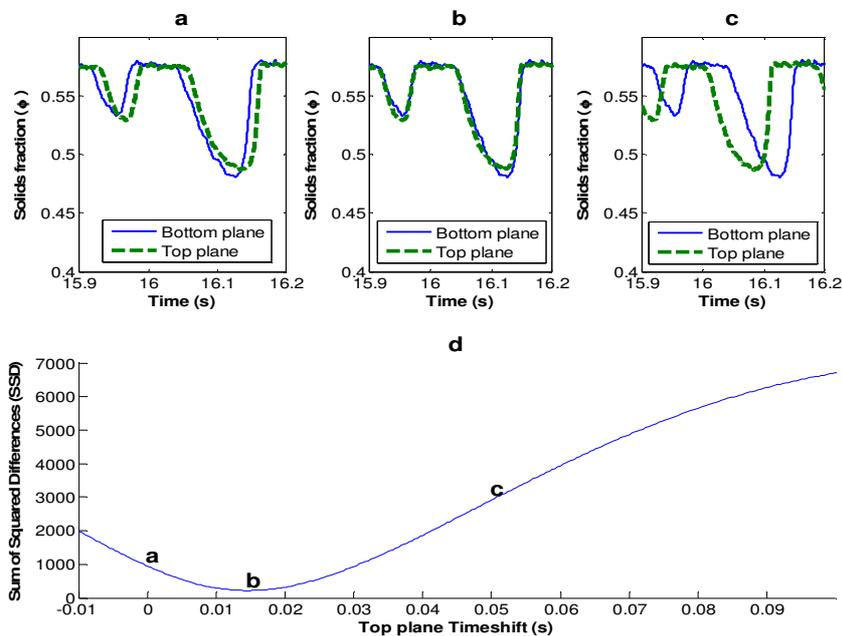
**Figure 1:** (a) is an example of the calculated cross sectional solids concentration signal obtained for both top and bottom measuring planes. The example is taken from the measurement done at 200mm above the distributor and at a velocity of 0.11 m/s. (b) and (c) shows the same signal, except the top plane's signal is shifted in time. (d) is the calculated SSD between the top and bottom plane signals at different top plane time shifts.
