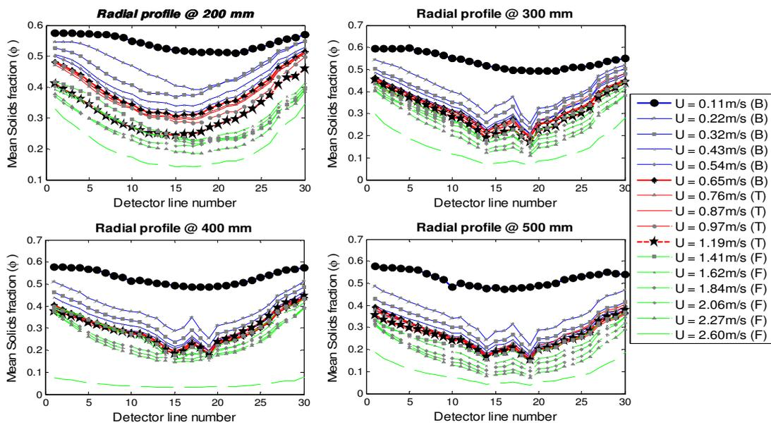
**Figure 4:** Radial solids distribution at different velocities and heights above the distributor. Indicated is the relevant regime at each velocity: "B" – bubbling regime, "T"–turbulent regime, "F" – fast fluidization regime.
