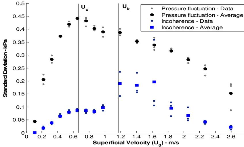
**Figure 2:** Standard deviation of pressure fluctuations, showing the bubbling to turbulent regime transition ( $U_c$ ) occurs at 0.65 m/s. The end of turbulent fluidisation ( $U_k$ ) is 1.19 m/s. Also shown is the standard deviation of incoherence, which is a measure of the void size.
