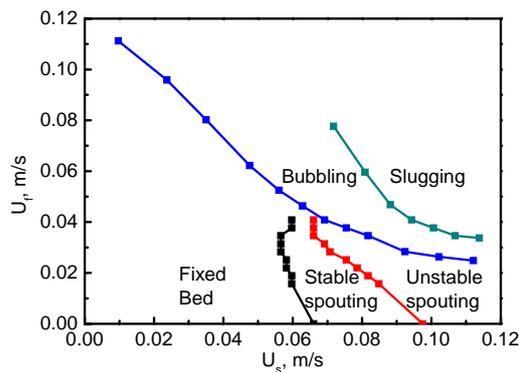
Fig. 2 Flow regime map for the conventional spout-fluid bed (Configuration A) at  $H=300$  mm,  $d_p=0.461$  mm,  $D_1=150$  mm
