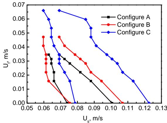
Fig. 6 Comparison of stable spouting regimes for the three spout-fluid bed configurations at  $H=350$  mm,  $d_p=0.461$  mm
