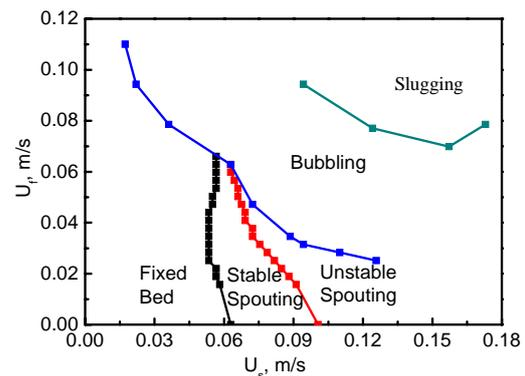
Fig. 3 Flow regime map for the spout-fluid bed with enlarged column (Configuration B) at  $H=300$  mm,  $d_p=0.461$  mm,  $D_1=150$  mm,  $D_2=170$  mm
