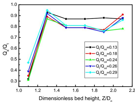
Fig. 7 Axial distribution of gas flow rate in the annular region in the conventional spout-fluid bed (Configuration A) at  $H=350$  mm,  $d_p=0.461$  mm,  $Q_s=4.8$  m<sup>3</sup>/h
