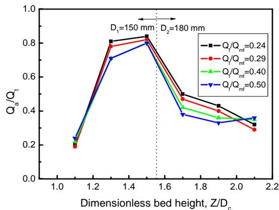
Fig. 9 Axial distribution of gas flow rate in the annular region in the spout-fluid bed with enlarged column (Configuration C) at  $H=350$  mm,  $d_p=0.461$  mm,  $D_1=150$  mm,  $D_2=180$  mm,  $Q_s=5.0$  m<sup>3</sup>/h
