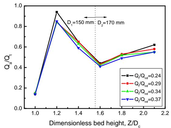
Fig. 8 Axial distribution of gas flow rate in the annular region in the spout-fluid bed with enlarged column (Configuration B) at  $H=350$  mm,  $d_p=0.461$  mm,  $D_1=150$  mm,  $D_2=170$  mm,  $Q_s=4.6$  m<sup>3</sup>/h
