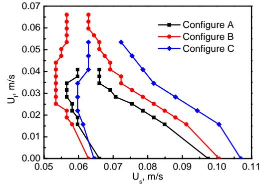
Fig. 5 Comparison of stable spouting regimes for the three spout-fluid bed configurations at  $H=300$  mm,  $d_p=0.461$  mm
