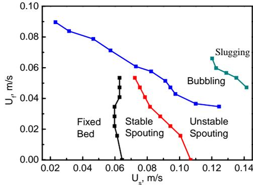
Fig. 4 Flow regime map for the spout-fluid bed with enlarged column (Configuration C) at  $H=300$  mm,  $d_p=0.461$  mm,  $D_1=150$  mm,  $D_2=180$  mm
