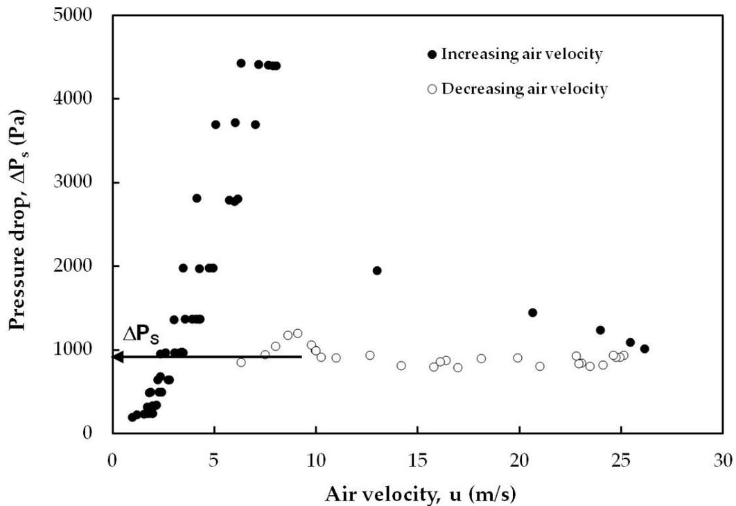
**Figure 4.** Evolution of the bed pressure drop with air velocity for a given system:  $d_p=0.002$  m;  $\gamma=36^\circ$ ;  $D_T=0.04$  m;  $W_H=0.025$  m;  $D_0=0.04$  m;  $H_0=0.14$  m
