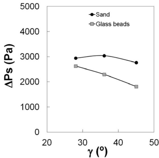
**Figure 7.** Influence of the contactor angle on the operating pressure drop.
