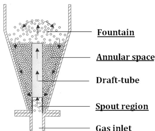
**Figure 1.** Zones in the conventional non-porous draft tube conical spouted bed.
