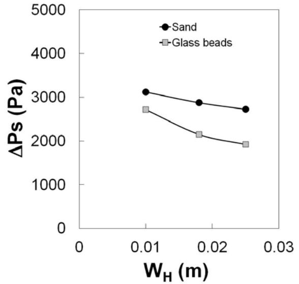
**Figure 6.** Influence of width of the faces on the operating pressure drop.
