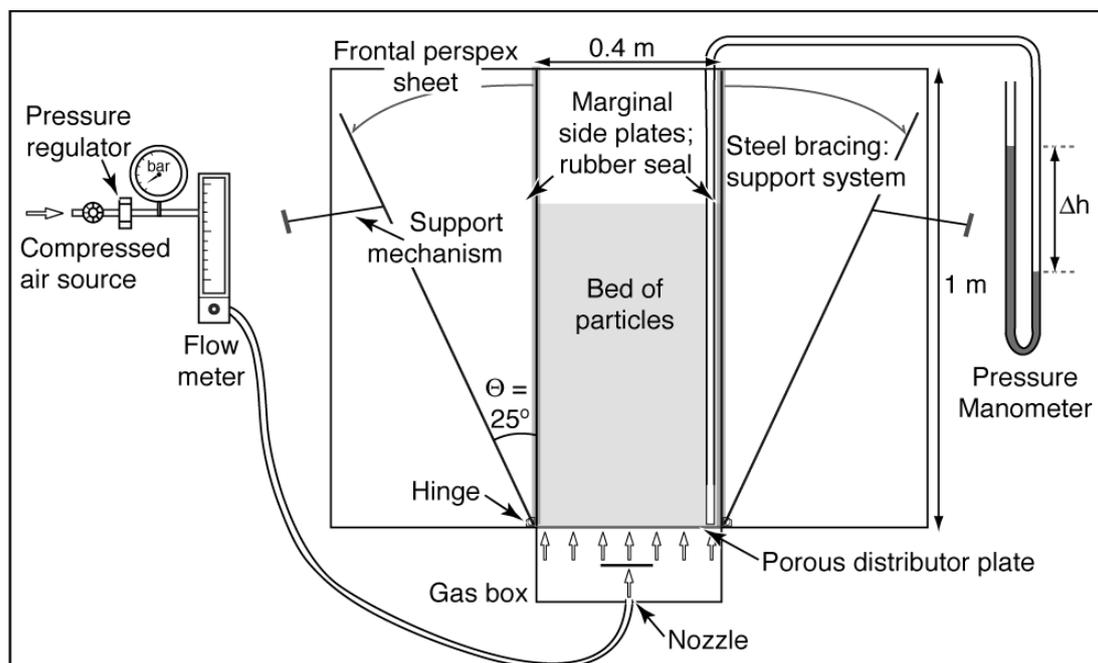
Figure 1. Schematic diagram of the experimental apparatus
