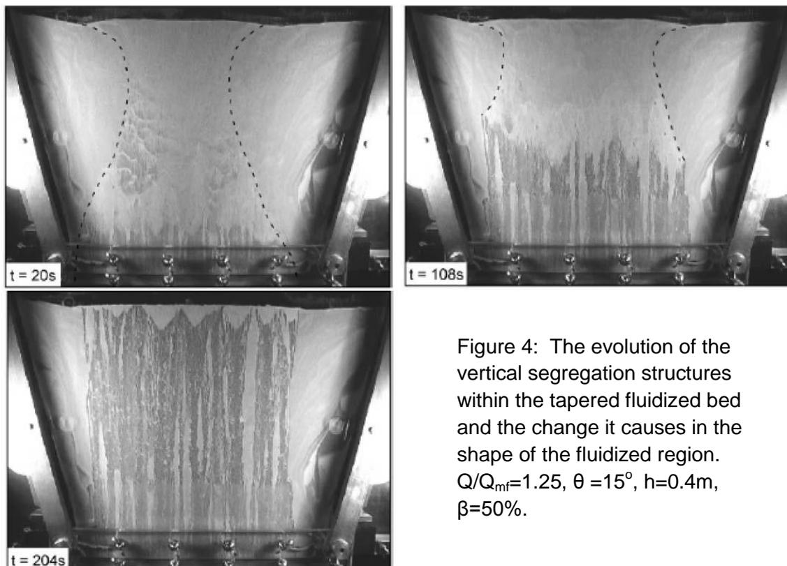
Figure 4: The evolution of the vertical segregation structures within the tapered fluidized bed and the change it causes in the shape of the fluidized region.  $Q/Q_{mf} = 1.25$ ,  $\theta = 15^\circ$ ,  $h = 0.4$  m,  $\beta = 50\%$ .
