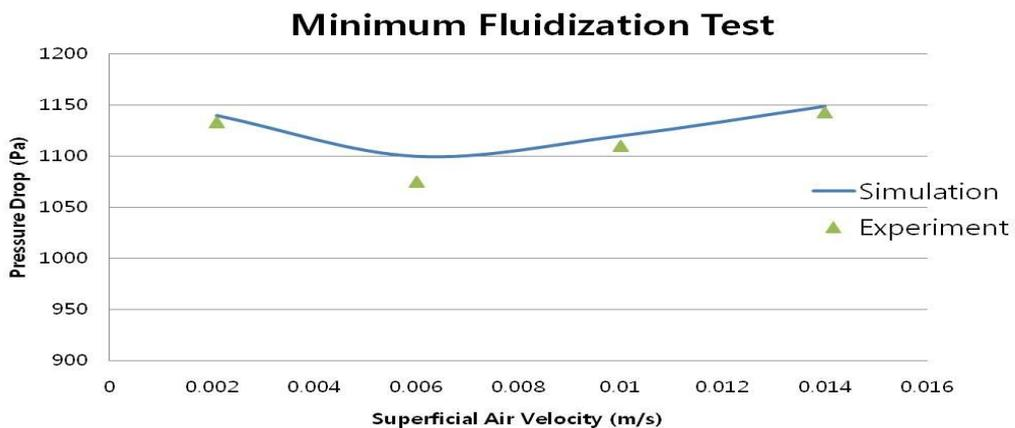
Figure 2. Comparison Between Our Simulation Results and PSRI/NETL Lab-scale Experimental Data
