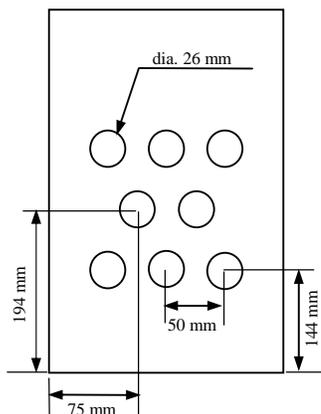
Figure 1. Geometry for the staggered arrangement. Drawing is not to scale.
