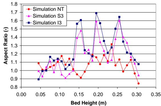
Figure 3. Bubble aspect ratio with bed height
