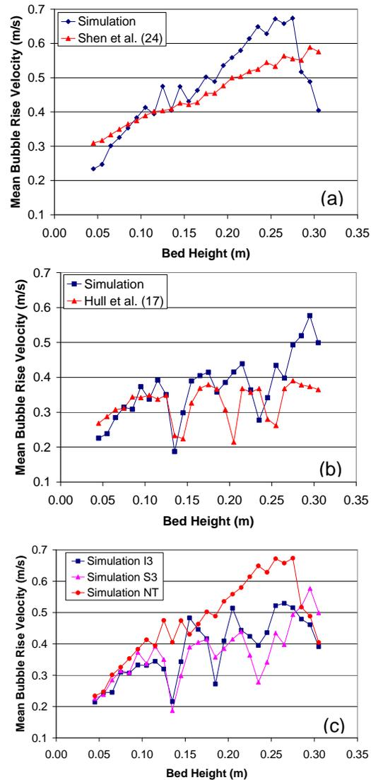
Figure 5. Mean bubble rise velocity versus bed height above distributor, (a) NT, (b) S3, (c) all
