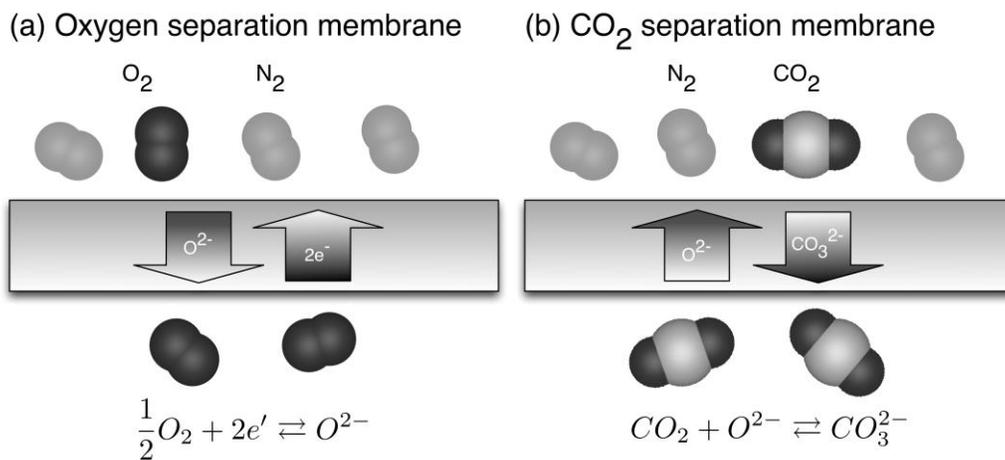
Figure 1 – Principles of (a) oxygen separation and (b) CO<sub>2</sub> separation membranes based on mixed conduction.
