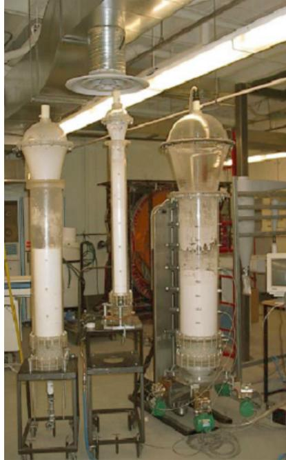
Figure 1. Experimental setup of fluidized bed columns
