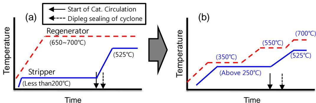
Fig. 6 Comparison of previous and new startup procedures
