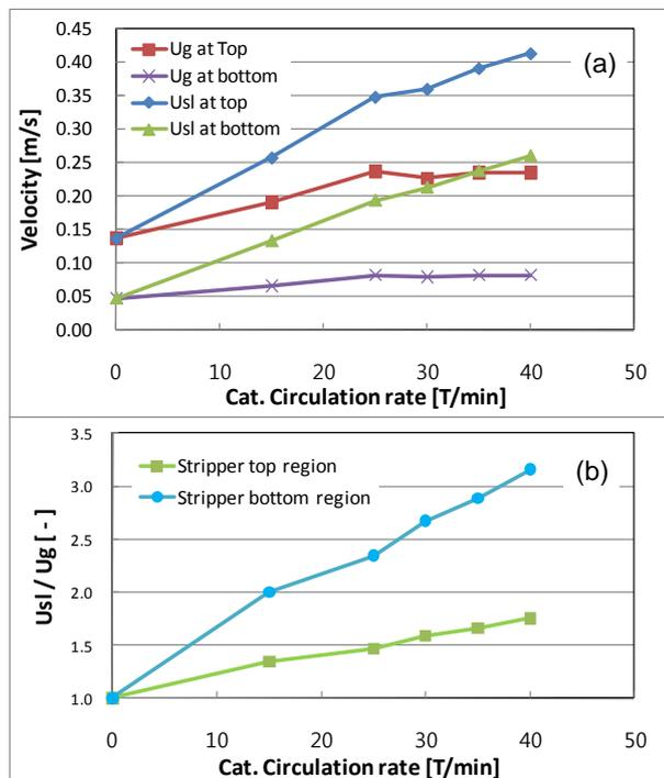
Fig. 5 (a) Effect of catalyst circulation rate on fluidizing velocity
