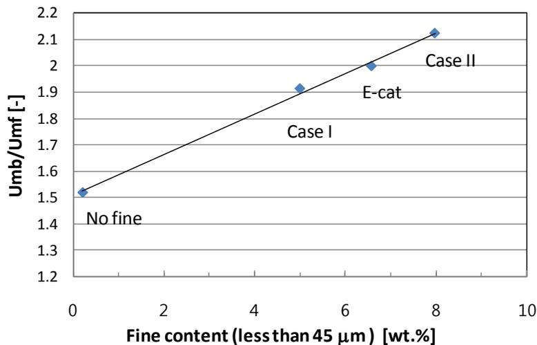
Fig. 4 Effect of fine content on catalyst fluidity
