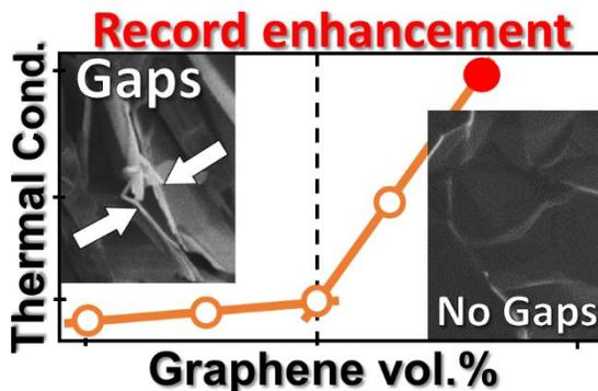
Figure 1 – Thermal conductivity enhancement via gap closure between adjacent fillers
