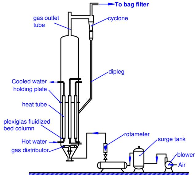
Figure 1 Schematic diagram of the experimental unit
