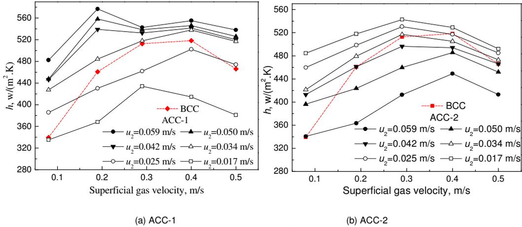
Figure 8 Bed-to-wall heat transfer coefficients of ACC-1 and ACC-2
