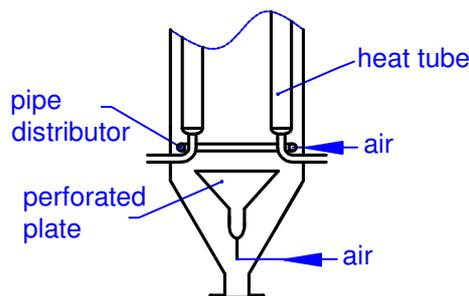
Figure 5 Gas distributors in annular catalyst coolers
