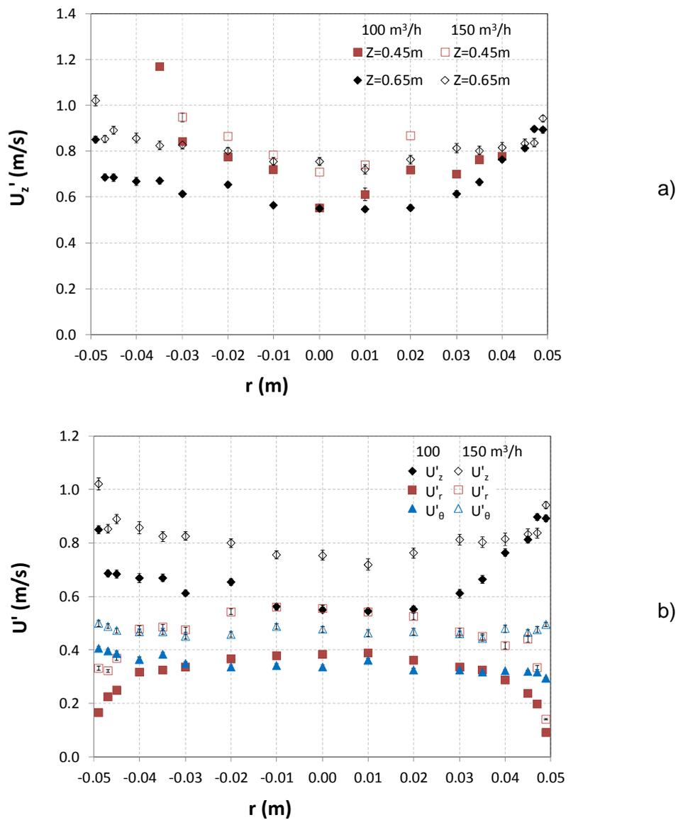
Figure 4: a) Axial solids velocity fluctuations and b) fluctuating solids velocity components at  $Z=0.65$  m ( $\delta=90^\circ$ , positive and negative  $r$  for  $\theta=270^\circ$  and  $\theta=90^\circ$  respectively, error bars for the 95% confidence intervals)
