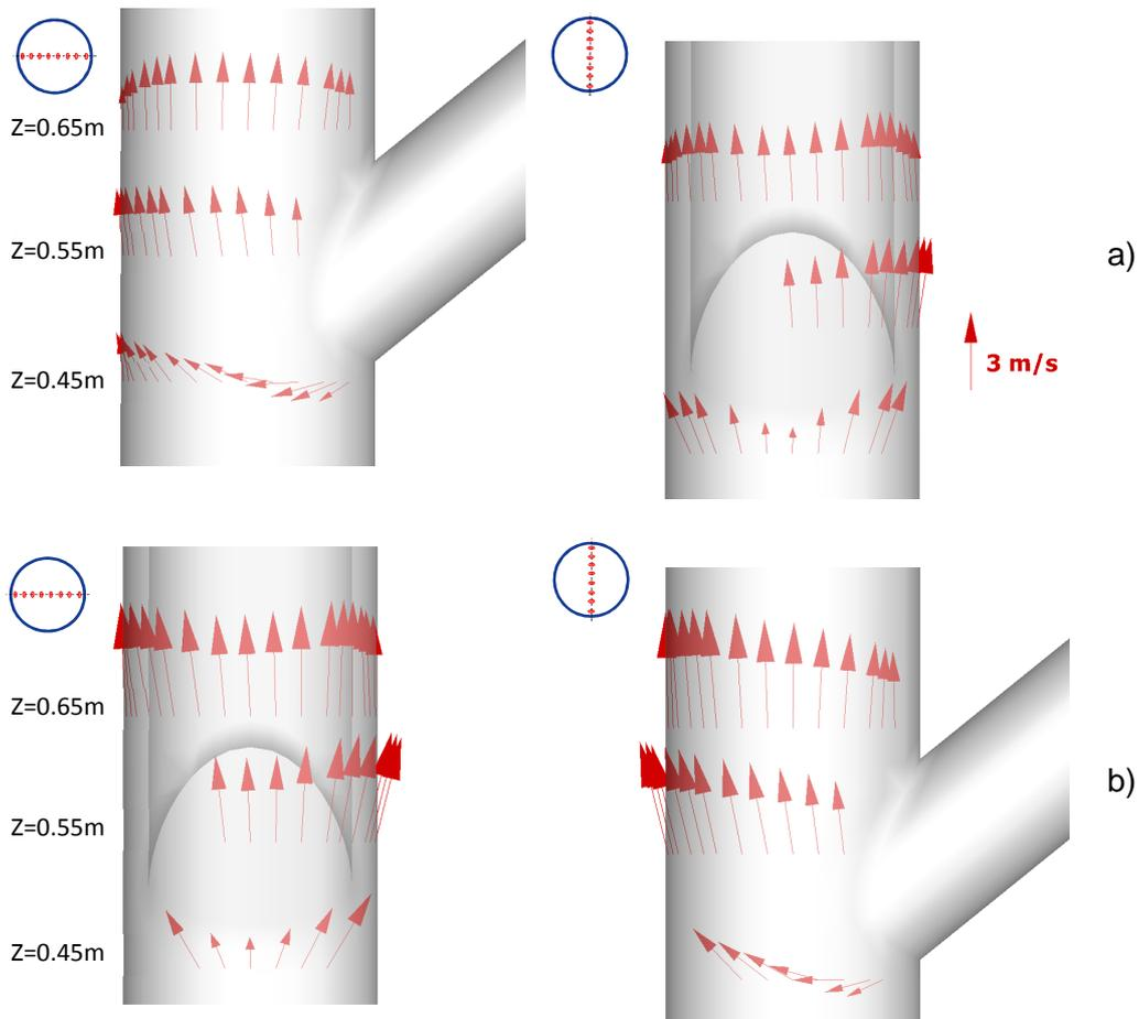
Figure 2: Side view of the riser flow for three riser heights, 0.45, 0.55 and 0.65 m and a) 100 m<sup>3</sup>/h and b) 150 m<sup>3</sup>/h gas flow.
