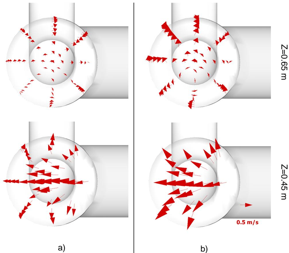
Figure 3: Top view of the riser flow for two riser heights,  $0.45$  and  $0.65$  m and a)  $100 \text{ m}^3/\text{h}$  and b)  $150 \text{ m}^3/\text{h}$  gas flow.
