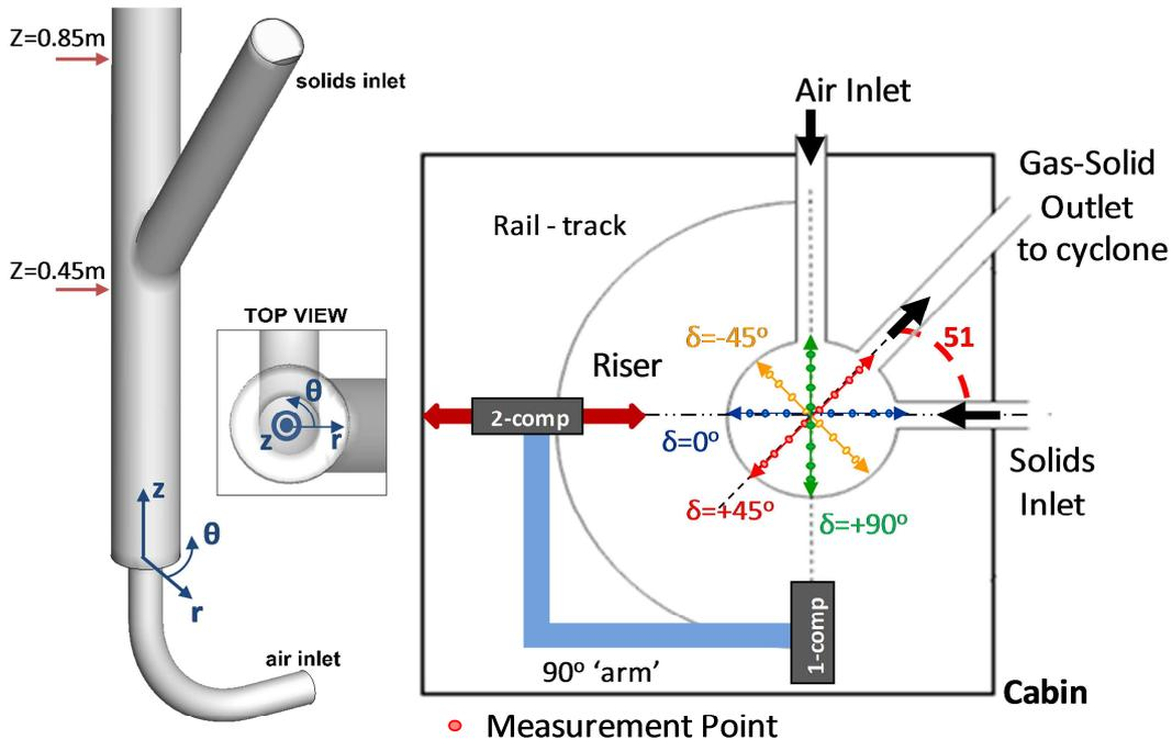
Figure 1: Riser inlet section and detail of the riser measurement section with a representation of the measuring planes.
