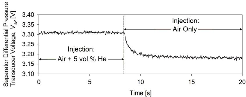
Figure 2 – Sample Separator Pressure Drop Signal
