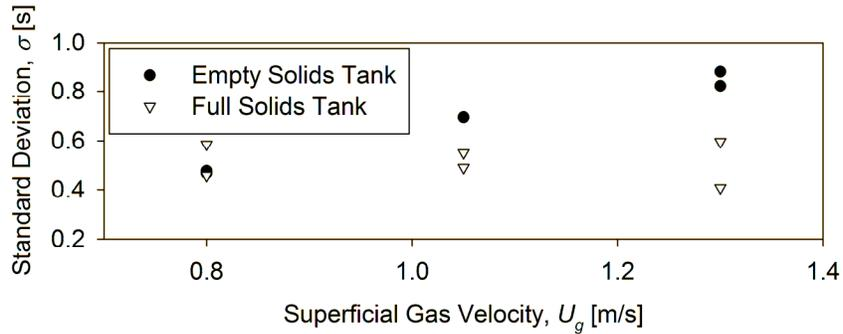
Figure 4 - Effect of Solids Tank Fill Level and Superficial Gas Velocity on Gas Backmixing (without solids)
