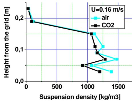
Figure 2. Distribution of solids concentrations for air and carbon dioxide velocities equal 0.01 m/s, 0.02 m/s, 0.04 m/s, 0.05 m/s, 0.07 m/s, 0.09 m/s, 0.11 m/s, 0.16 m/s, respectively.
