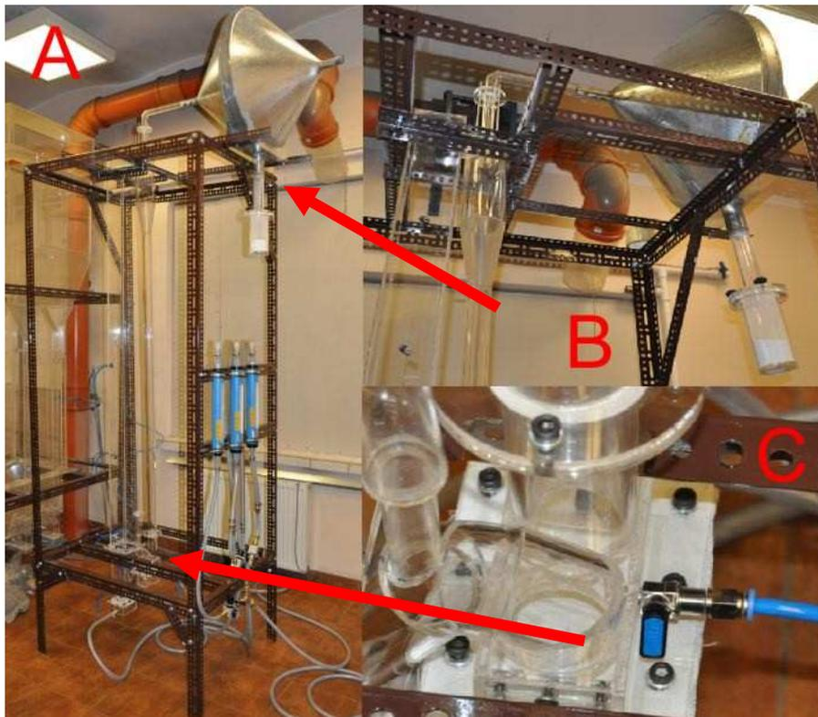
Figure 1. a) 3D cold model plexiglass circulating fluidized bed installation; b) cyclone and expansion tank; c) non-mechanical syphone and port for circulating glass beads collecting.
