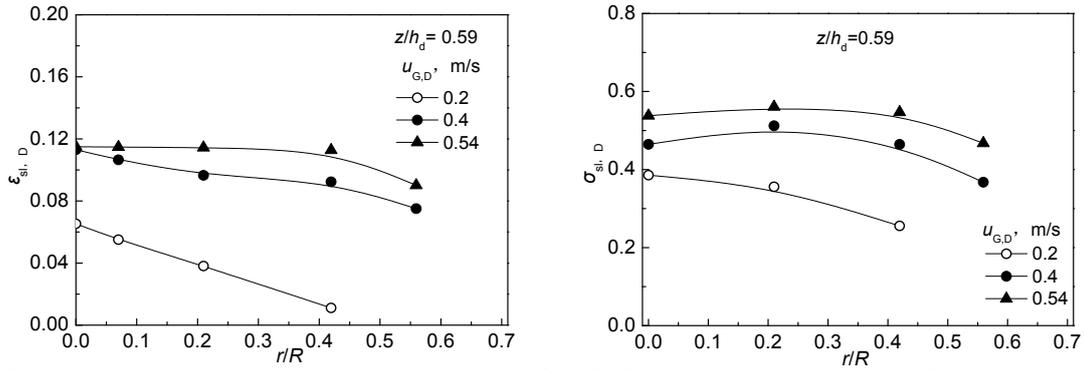
Fig. 5 Mean solid holdup and standard deviation of PDF of the bubble phase in the draft tube region
