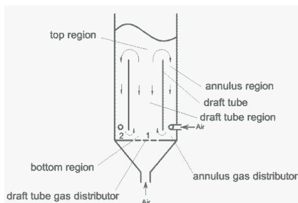
Fig.1 Schematic diagram of gas-solid airlift loop reactor
