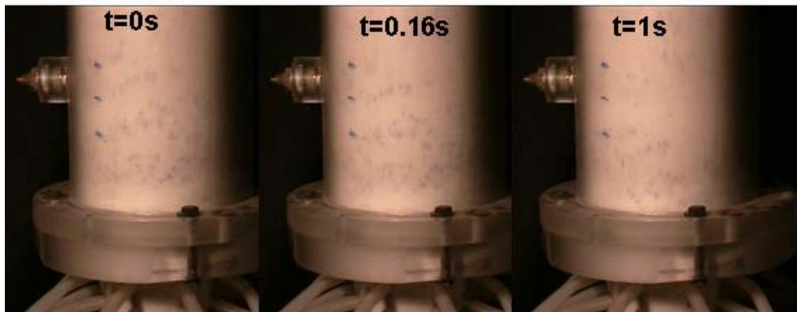
Figure 3 – Wall trajectory of some char particles obtained at different times. Bed material: alumina (150-200  $\mu\text{m}$ ); fluidization velocity: 0.17 m/s ( $U-U_{mf}=0.16$  m/s, bed inventory=1.95 kg).
