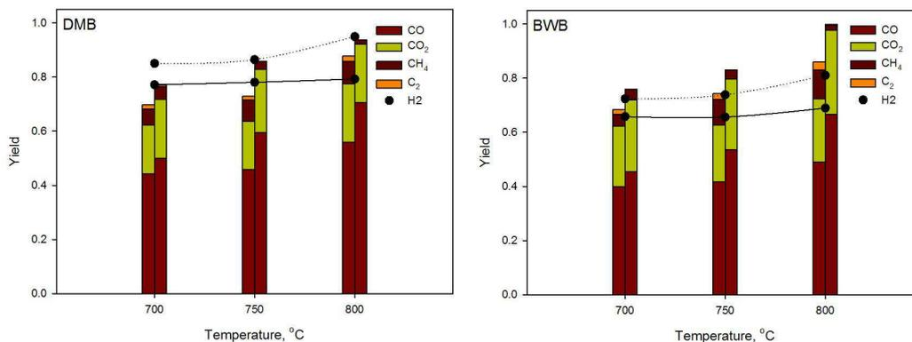
Figure 6. Yield of product gases from catalytic cracking of the DMB and the BWB versus temperature. Residence time= 30s; left hand side bars: mass of the catalyst  $X= 0.5$  g; right hand side bars: mass of the catalyst  $X= 1$  g.
