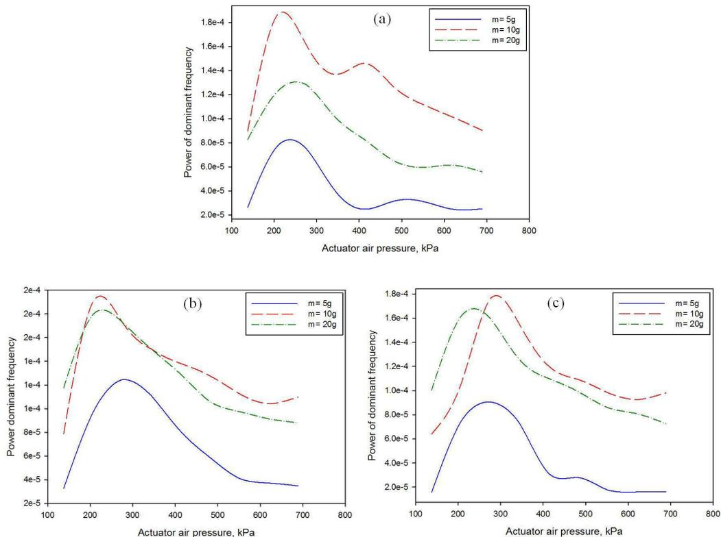
Figure 4. Effect of mass of the particles on dominant frequency power of the particle mixing; sand particles with size of (a) 212-355  $\mu\text{m}$ , (b) 149-212  $\mu\text{m}$  and (c) 75-149  $\mu\text{m}$
