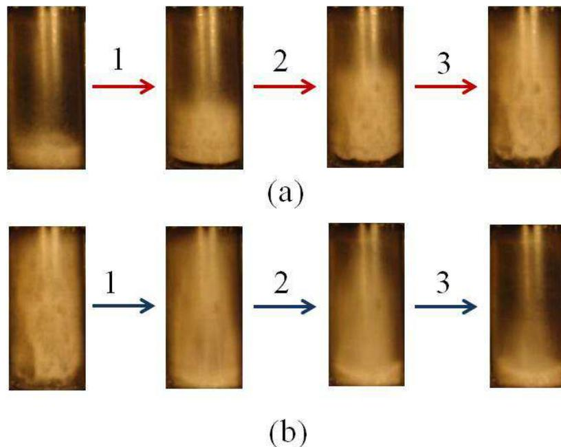
Figure 2. Sequences of mixing of catalyst particles in the jiggle bed reactor: (a) bed expansion during downward actuator retraction (b) bed contraction during upward actuator extension.
