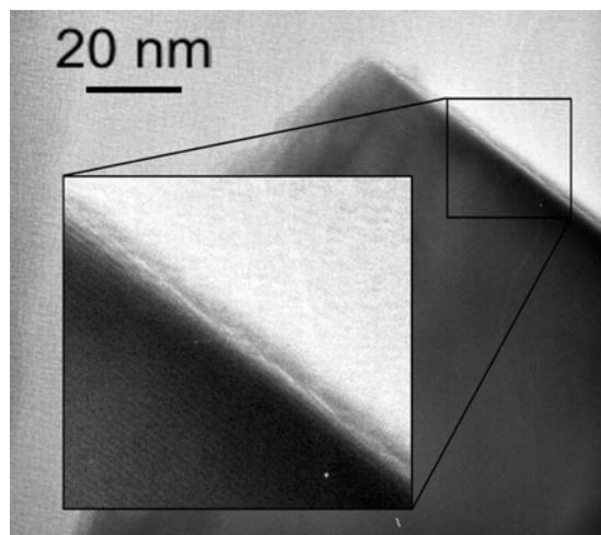
**Figure 2.** TEM picture of a  $\text{LiMn}_2\text{O}_4$  particle coated with a thin layer of alumina (five ALD cycles) at atmospheric pressure. Such nanoparticles can be used as cathode material in Li-ion batteries (8).
