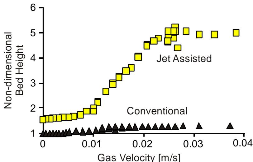
**Figure 3.** Comparison of the non-dimensional fluidized bed height as a function of gas velocity for conventional and microjet assisted fluidization of Aerioxide  $\text{TiO}_2$  P25 (ABF nanopowder) in a 12.7 cm diameter column. The jet diameter is 254  $\mu\text{m}$ , and the jet velocity is 320 m/s.
