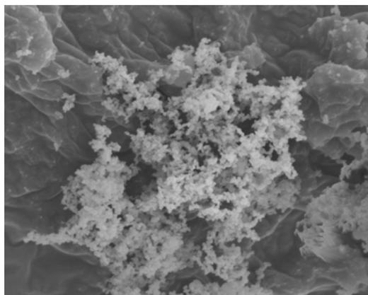
**Figure 1.** SEM image of agglomerate of silica nanoparticles.
