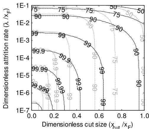
**Figure 2: Model 1 and Model 0 results compared. The gray contours represent  $\eta_0$  while the black contours represent  $\eta_1$ , both for typical values of  $\sigma_g = 1.4$  and  $\beta = 6.0$ . Both efficiencies read in percent.**
