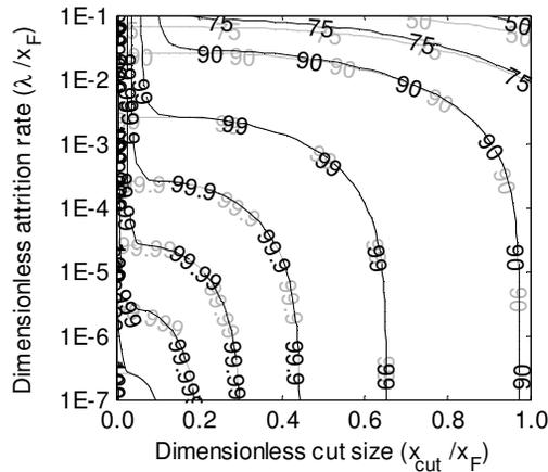
**Figure 4: Model 3 (natural PSD with median  $0.1x_F$  and  $\sigma_g = 1.4$ ) and Model 1 results compared. The gray contours represent  $\eta_1$  while the black contours represent  $\eta_3$ , both for typical values of  $\sigma_g = 1.4$  and  $\beta = 6.0$ . Both efficiencies read in percent.**
