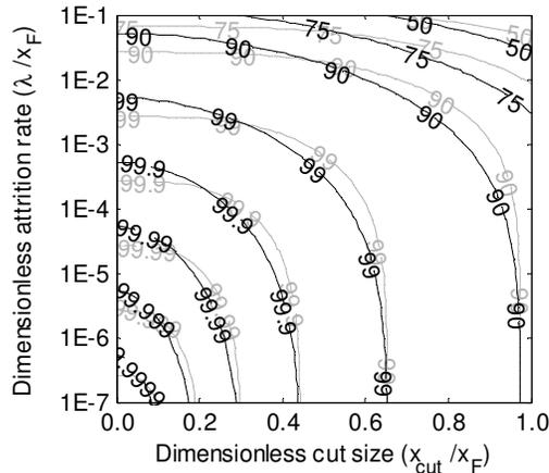
**Figure 3: Model 2 (for  $n = 2$ ) and Model 1 results compared. The gray contours represent  $\eta_1$  while the black contours represent  $\eta_2$ , both for typical values of  $\sigma_g = 1.4$  and  $\beta = 6.0$ . Both efficiencies read in percent.**
