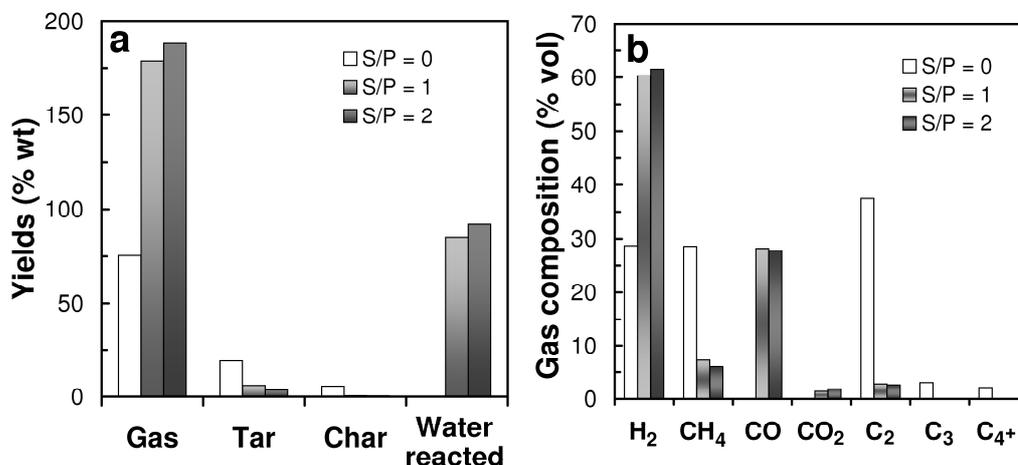
**Figure 3** Effect of S/P ratio on product yields for 100 g of plastic fed into the reactor (Figure 3a) and on gas fraction composition (Figure 3b).
