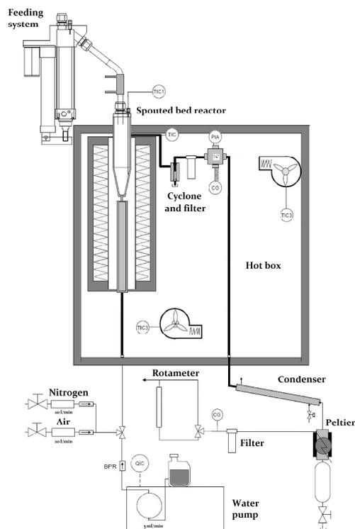
**Figure 1.** Scheme of the laboratory scale plant.
