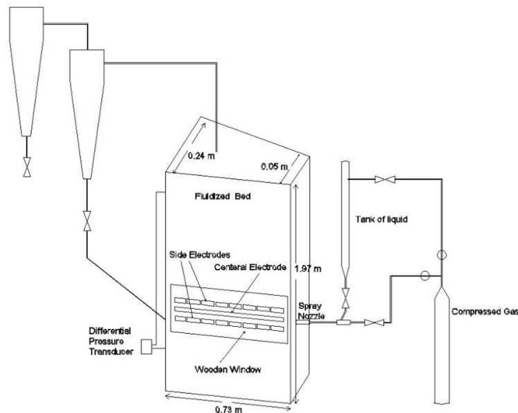
Figure 1 - Schematic of experimental set up
