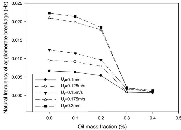
Figure 3 - Effects of fluidization velocity and oil mass fraction on natural frequency of agglomerate breakage
