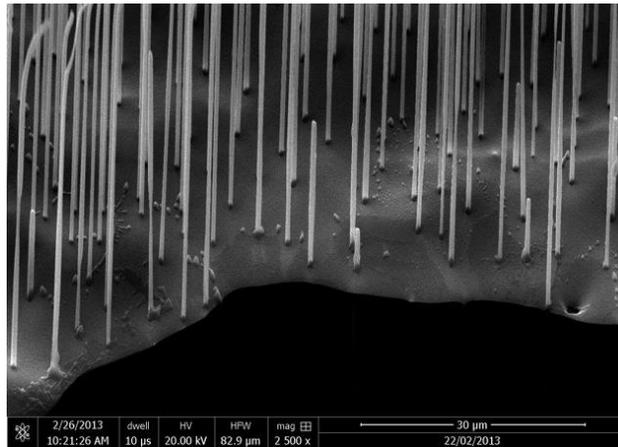
Figure 1 – Be wires obtained after etching away the Al matrix of an Al/Be eutectic alloy (SEM image).
