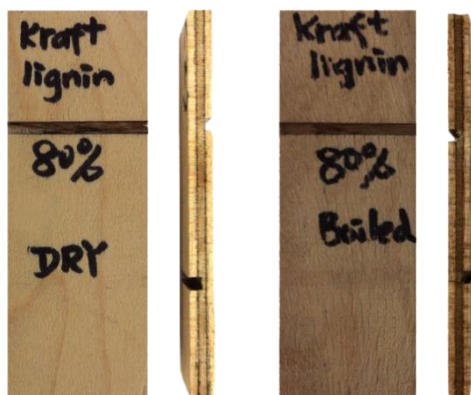
Figure 1 – Plywood panels bonded with bio-phenol adhesives (80% of phenol substitution by kraft lignin pyrolysis bio-oils).
