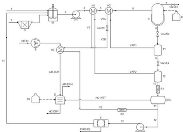
Figure 1: schematic flow sheet of the HTC plant.
