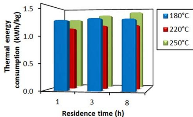
Figure 2: specific thermal energy consumption (kWh/kg<sub>char</sub>) at different HTC temperatures (180, 220, 250 °C) and residence times (1, 3, 8 h; data refers to HTC of grape marc with B/W=0.19).
