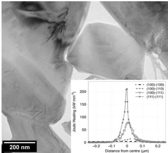
Figure 1 – TEM micrograph of FLASH sintered KNN, with amorphized GBs and penetration of sharp edge through neighbor face. Overlapped calculated Joule heating for the four considered possible particle contacts.
