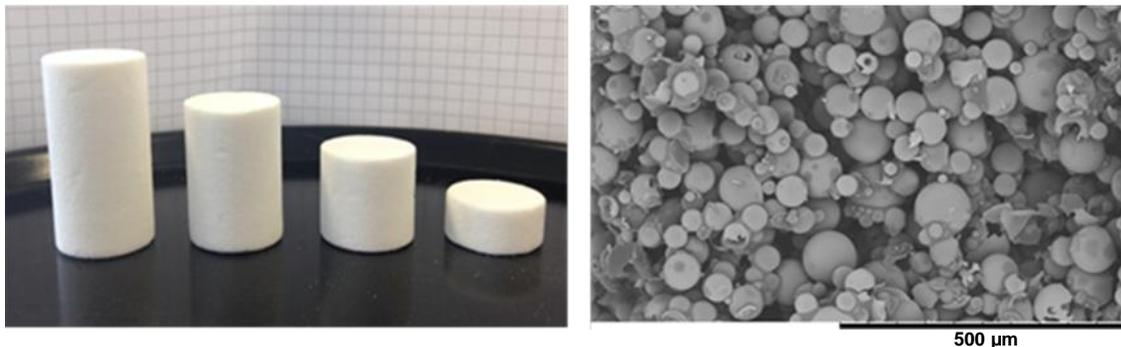
Figure 1 – Final parts prepared using optimized SLS protocol (cylinders with the 20 mm diameter and height: 40, 30, 20 and 10 mm) with the detail SEM image of the final part structure.
