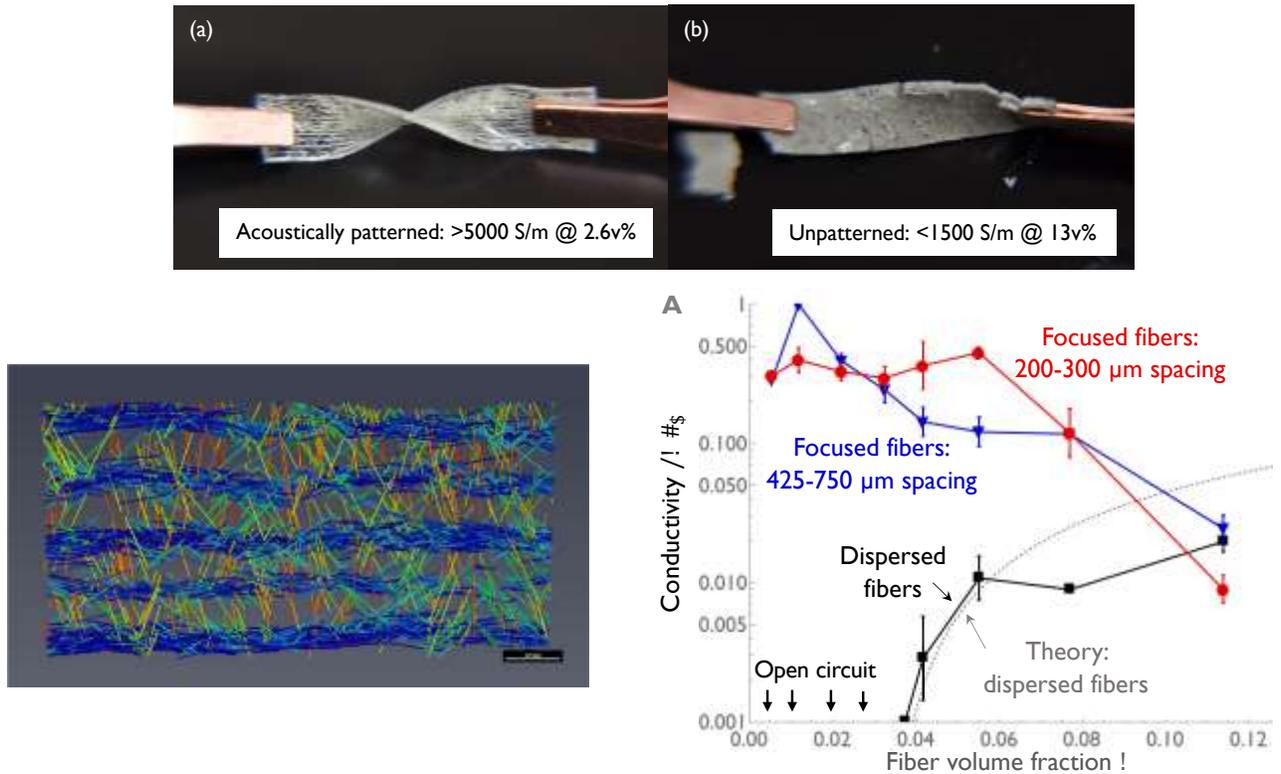
Figure 1 – Acoustic focusing allows on-the-fly alignment of conductivity particles, leading to (i) strong conductivity at volume fractions well below the percolation threshold (ii) decoupling between the mechanical properties of the matrix and particles.
