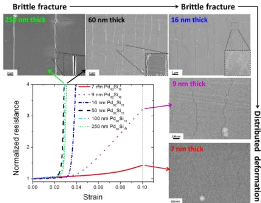
Fig. 1. Overview of electro-mechanical behavior of thin metallic glass films on polymer substrate
