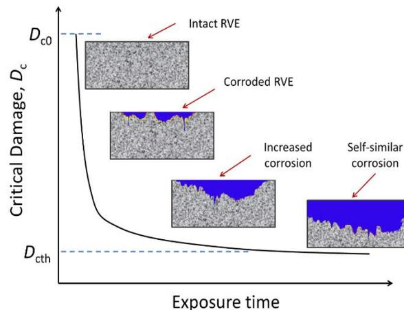
Figure 1 – A schematic that shows the concept of corroded RVE. The critical damage changes from  $D_{c0}$  for un-corroded RVE to  $D_{cth}$  for self-similar corroded RVE.
